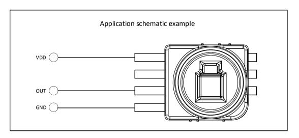
*Figure 9: Basic application example with pin 1 as GND*
