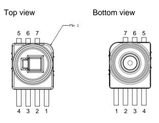
Figure 3: Package pinout
