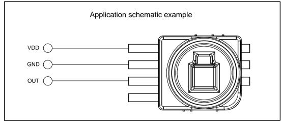
Figure 8: Basic application example with pin 3 as GND
