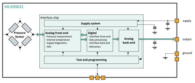
Figure 5: MLX90822 block diagram
