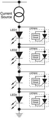
Note: The interaction between the Bourns® LSP device and the power supply for the LED series string dictates the power supply architecture. Proper care must be taken in the design of the power supply architecture to ensure that the Bourns® LSP devices operate as intended and the design maintains integrity.
