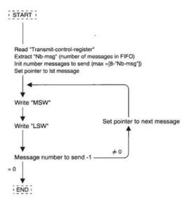
Figure 35. Transmitter with Interrupt Flow-chart
