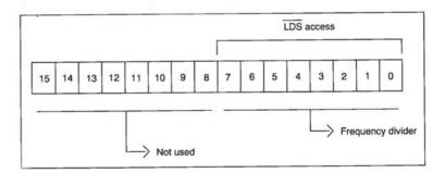
The transmission frequency can be computed by dividing the CLK ARINC frequency by the frequency register value.
