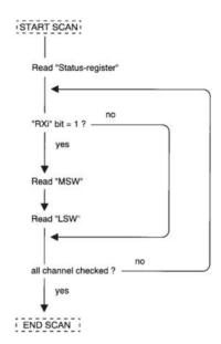
Figure 33. Receiver with Interrupt Flow-chart
