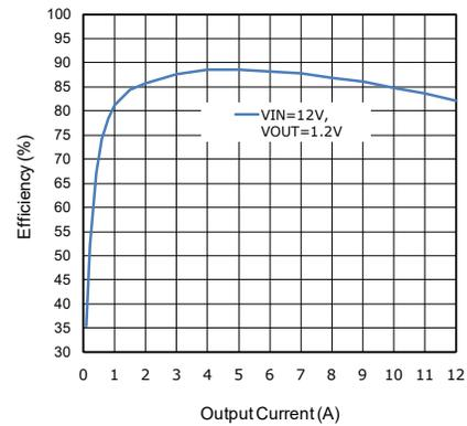
Fig. 15: Efficiency versus  $I_{OUT}$ ,  $V_{IN}=12V$ ,  $V_{OUT}=1.2$
