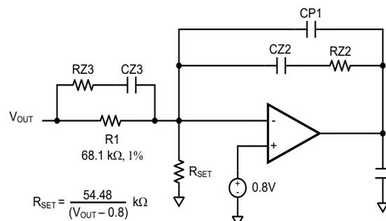
Fig. 24: Type III Error Amplifier Compensation Circuit
