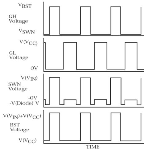
The second feature is a 100% duty cycle timeout that ensures synchronized refreshing of the BST capacitor at very high duty ratios. In the event that the high side NFET is on for 20 continuous clock cycles, a reset is given to the PWM flip flop half way through the 21<sup>st</sup> cycle. This forces GL to rise for the cycle, in turn refreshing the BST capacitor. The boost capacitor is used to generate a high voltage drive supply for the high side switch, which is  $V_{CC}$  above  $V_{IN}$ .
