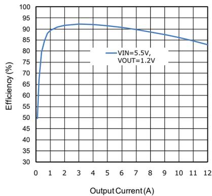
Fig. 14: Efficiency versus  $I_{OUT}$ ,  $V_{IN}=5.5V$ ,  $V_{OUT}=1.2$
