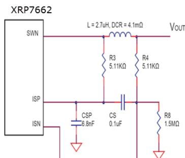
Fig. 21: Over Current Detection Circuit for  $I_{MAX} < (60mV/DCR)$
