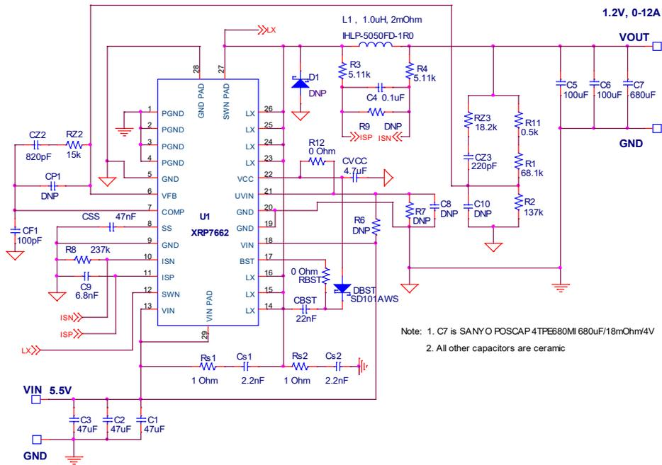
Fig. 16: 5.5V<sub>IN</sub> test circuit
