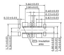
Recommended metal mask pattern Metal mask thickness: When 100 µm (Power contact opening ratio: 71%) (Terminal opening ratio: 75%) (Metal-part opening ratio: 100%)
