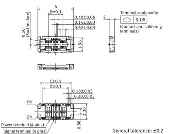
\*\*Because the soldering terminal Y and Z are the unified structure, they are connected electrically.
