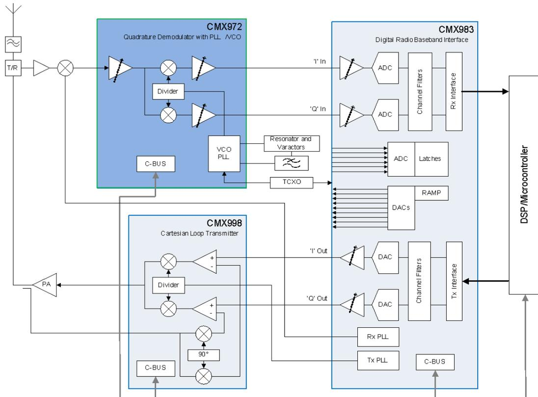
Figure 5. Typical system application utilising CMX972 Quadrature Demodulator with PLL/VCO, CMX998 Cartesian Feedback Loop Tx and CMX983 AFE Digital Radio Interface IC.
