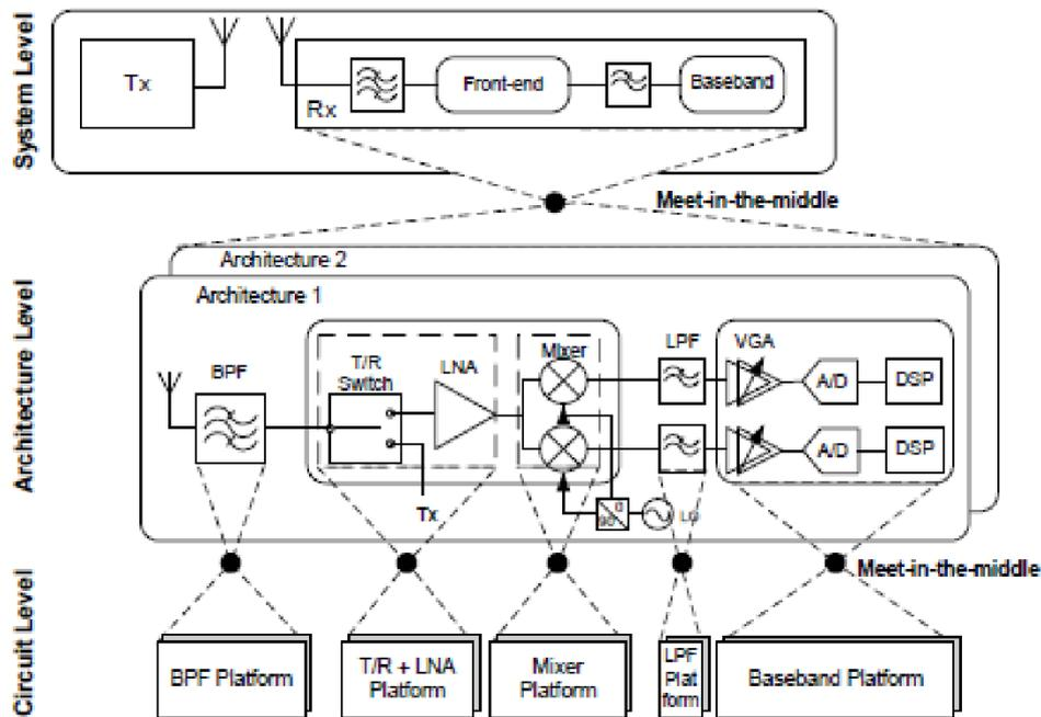
Figure 2. Platform-based approach to transceiver design.
