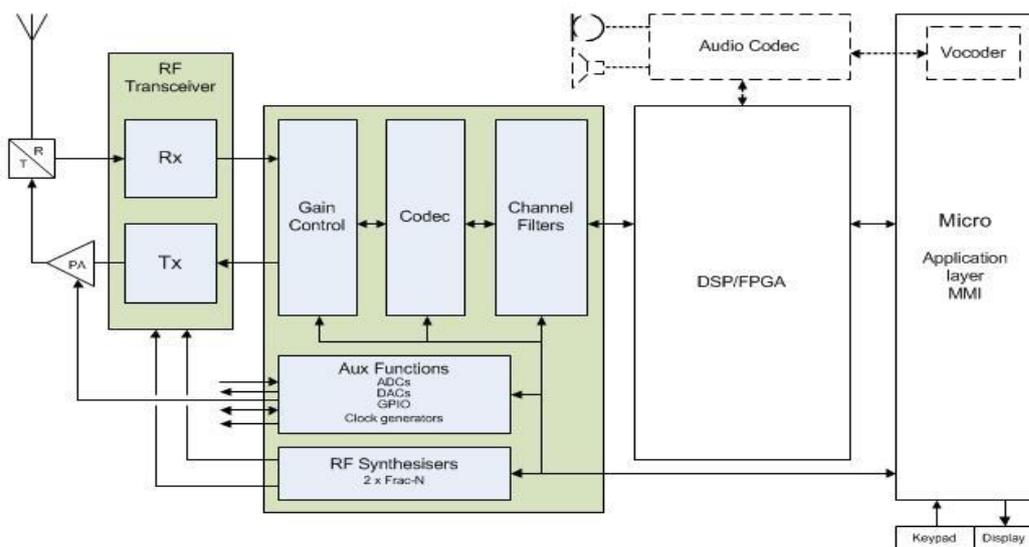
Figure 3. Typical system architectures for building block RF designs.
