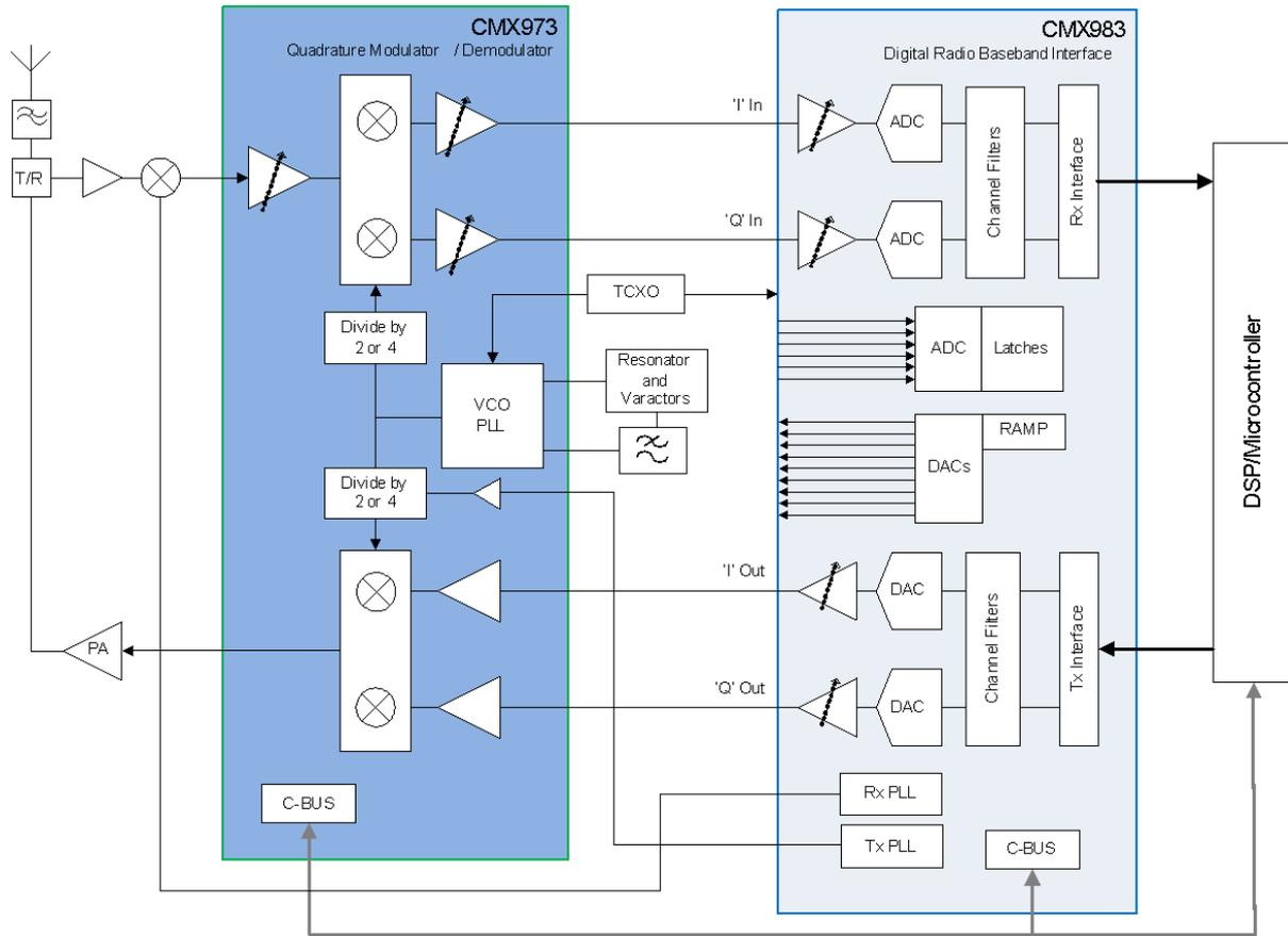
Figure 6. Typical system application utilising CMX973 Quadrature Modulator/Demodulator and CMX983 AFE Digital Radio Interface.
