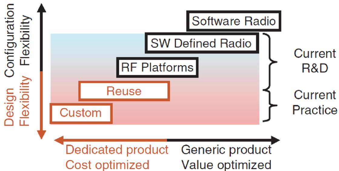
Figure 1. Platform-based RF system design (Source: Peter Baltus – Philips Semiconductors and Eindhoven University).
