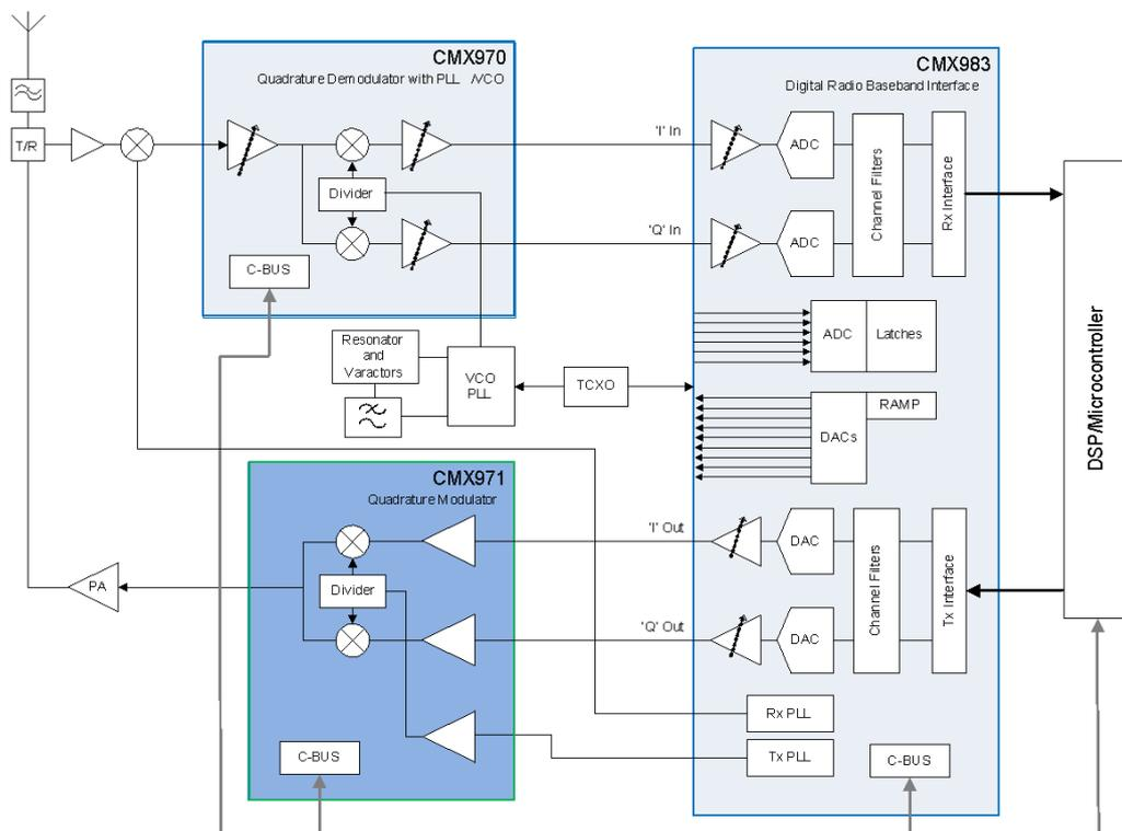
Figure 4. Typical system application utilising CMX971 Quadrature Demodulator, CMX970 IF/RF Quadrature Demodulator and CMX983 Programmable Baseband Interface IC.
