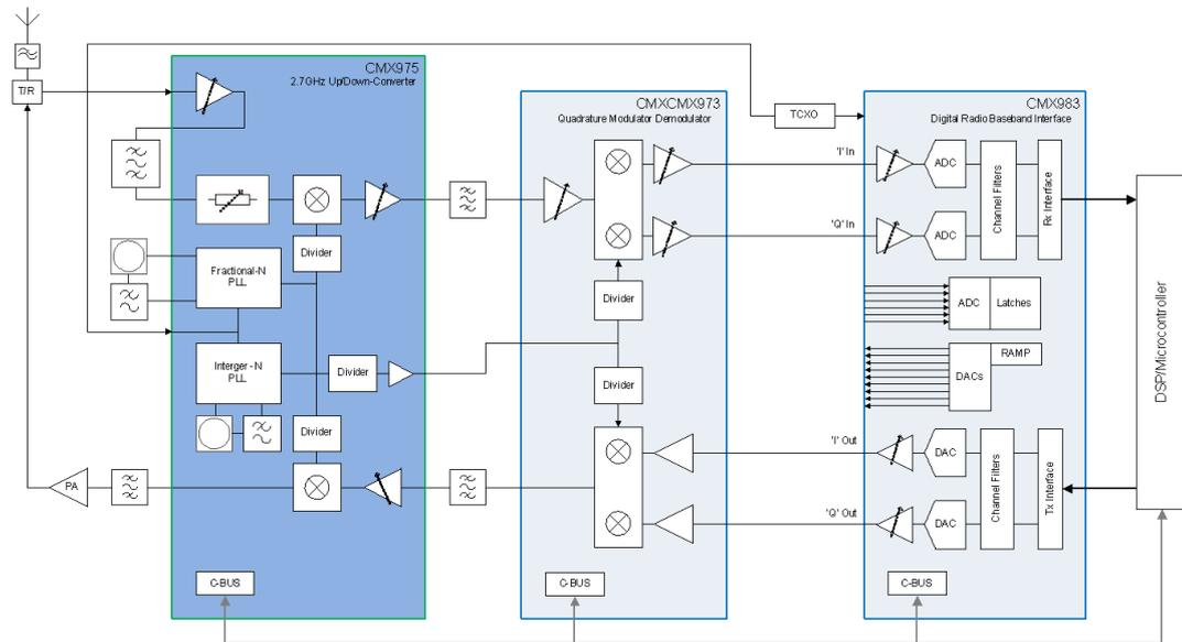
Figure 7. The CMX975 has been designed to work with CML's CMX973 Quadrature Modulator/Demodulator to provide a simple and cost effective high frequency superheterodyne transceiver operating in the range 1 to 2.7 GHz.
