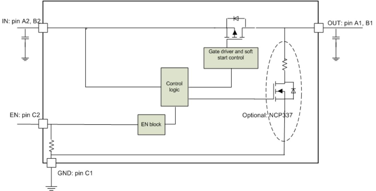
**Figure 2. Block Diagram**
