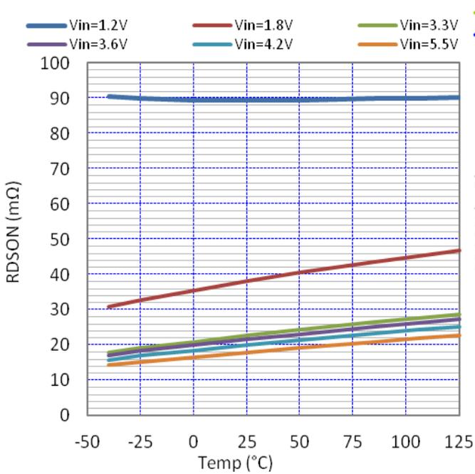
Figure 6. Rdson (mΩ) vs. Temperature (°C) at 100 mA
