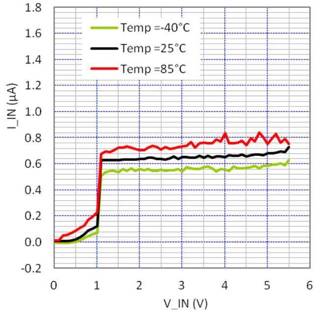
Figure 11. Quiescent Current ( $\mu\text{A}$ ) vs. Temperature ( $^{\circ}\text{C}$ )
