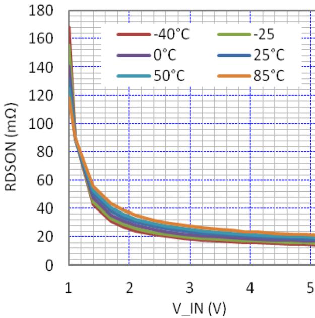
Figure 4. Rdson (mΩ) vs. Vin (V)
