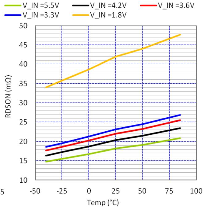
Figure 7. Rdson (mΩ) vs. Temperature (°C) at 3 A
