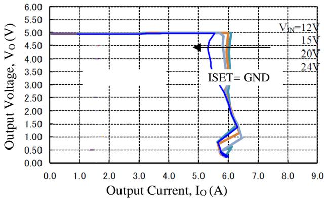
Figure 4-5. Overcurrent Protection
