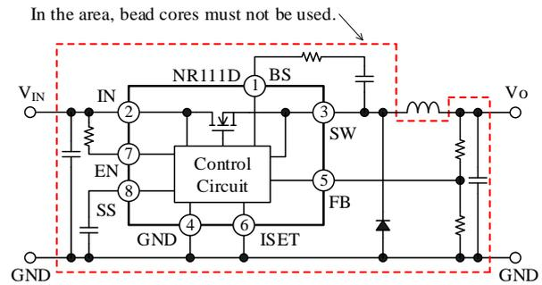
Figure 11-10. Note when you add bead cores
