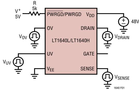
Figure 1. Test Circuit
