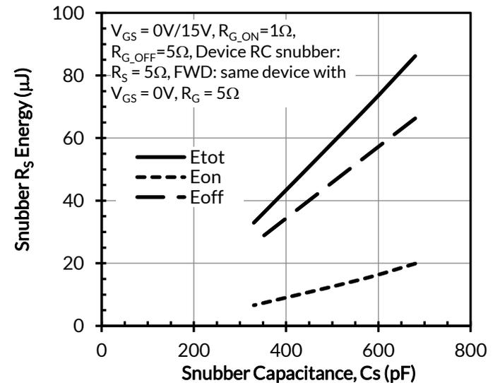
Figure 23. Clamped inductive switching energy vs. Snubber Capacitance  $C_S$  at  $V_{DS} = 400V$ ,  $I_D = 70A$ , and  $T_J = 25^\circ C$
