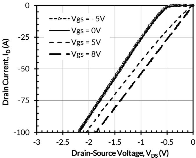
Figure 11. 3rd quadrant characteristics at  $T_j = 175^\circ\text{C}$
