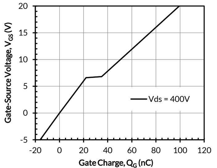
Figure 8. Typical gate charge at  $I_D = 70A$
