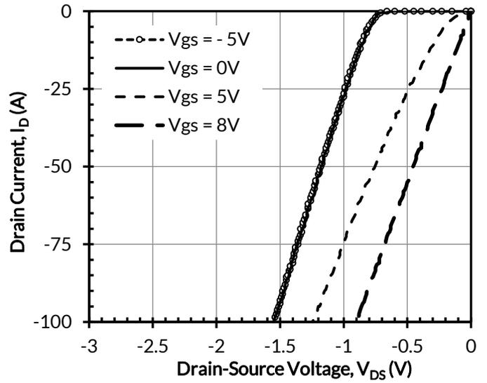
Figure 10. 3rd quadrant characteristics at  $T_j = 25^\circ\text{C}$
