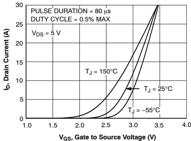
Figure 5. Transfer Characteristics
