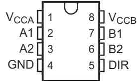
**Figure 5-1. DCU Package, 5-Pin VSSOP (Top View)**
