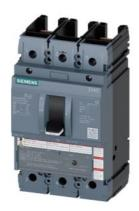
circuit breaker 3VA5 UL frame 250 breaking capacity class C 100kA @ 480V 2-pole, line protection TM230, FTAM, In=80A overload protection Ir=80A fixed short-circuit protection li=5...10 x In without connection
