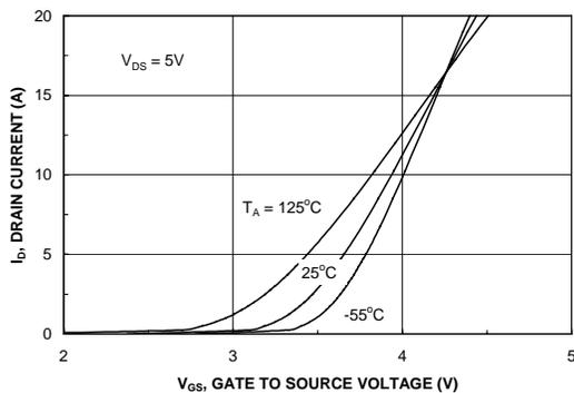
Figure 5. Transfer Characteristics.
