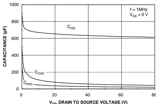
Figure 8. Capacitance Characteristics.
