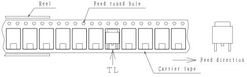
Those with one electrode terminal on the feed hole side · · · · · TL
