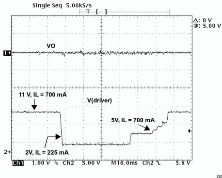
Figure 13. Input Voltage Excursions (Similar to Low-Crank Conditions)
