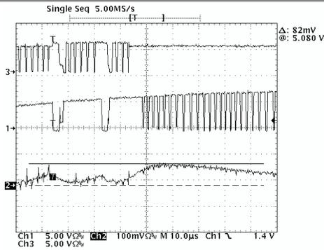
Figure 15. Switch-Mode Regulator Transition From Boost Mode to Buck Mode
