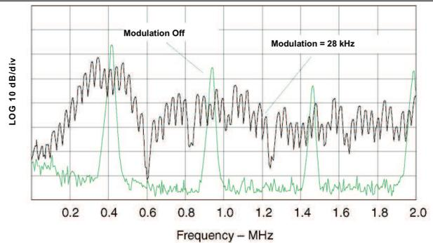
These values represent conducted EMI results of a test board for display purposes only. Actual results may vary greatly depending on board layout and external components and must be verified in actual application.
