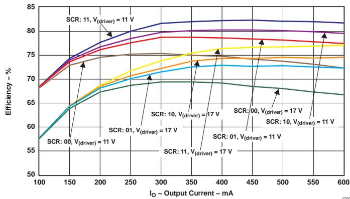
NOTE: The average converter efficiency with four different slew rate controls (SCRx) on the Q1 switching FET with input voltage  $V_{(driver)} = 11\text{ V}$  and  $17\text{ V}$ ,  $T_A = 125^\circ\text{C}$ .
