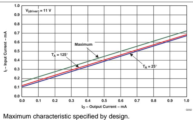
Figure 2. Low-Power-Mode Current,  $I_O = 0 \text{ mA} - 1 \text{ mA}$
