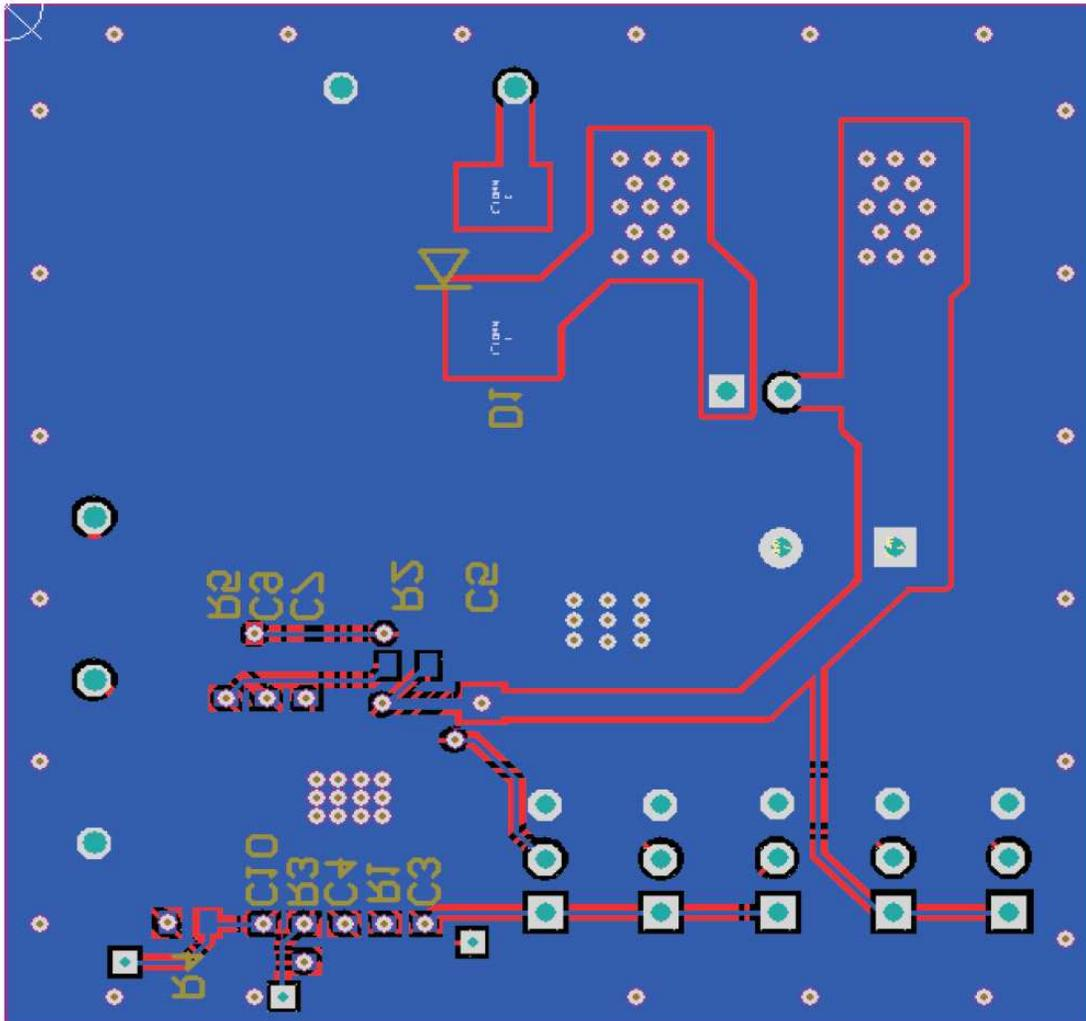
Large ground plane to reduce noise and ground-loop errors
