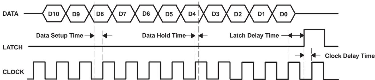
NOTE: Data is clocked in on the positive edge of the clock. The positive edge of the latch signal should occur before the next positive edge of the clock. For definition of D0 to D10, see the control logic table.
