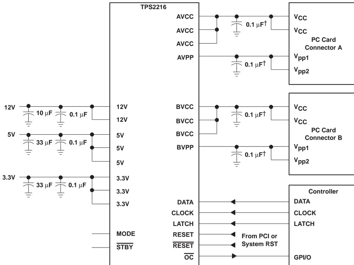
† Maximum recommended output capacitance for xVCC is 220  $\mu$ F and for xVPP is 10  $\mu$ F without  $\overline{\text{OC}}$  glitch when switches are powered on.
