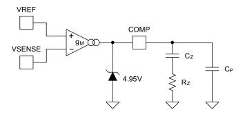
Figure 27. Transconductance Error Amplifier With Typical Compensation Network
