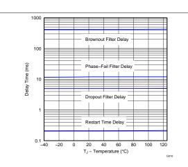
Figure 21. Various Delay Times vs Temperature
