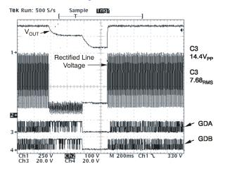
Figure 38. UCC28063A Response to a Line Brownout Event at 265 V<sub>RMS</sub>
