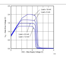
Figure 20. Gate Drive Low Voltage in UVLO vs Bias Supply Voltage
