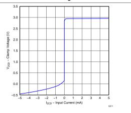
Figure 22. Zero Current Detect Clamp Voltage vs Input Current
