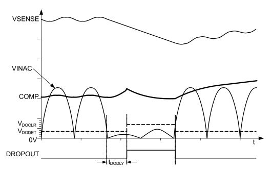
Figure 32. AC-Line Dropout Timing With Illustrative System Behavior
