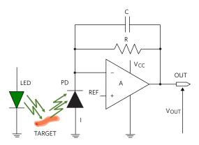
Figure 3. The transimpedance amplifer
