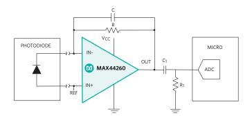
Figure 4. Signal processing
