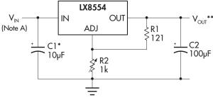
\* Needed if device is far from filter capacitors.
