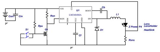
FIGURE 1. Example Schematic Showing Connection for all Components.
