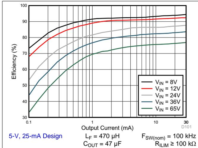
Figure 1. Converter Efficiency: 5 V, 25 mA, PFM
