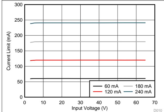
Figure 15. Peak Current Limits vs Input Voltage
