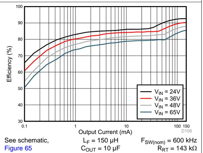
Figure 6. Converter Efficiency: 15 V, 150 mA, COT
