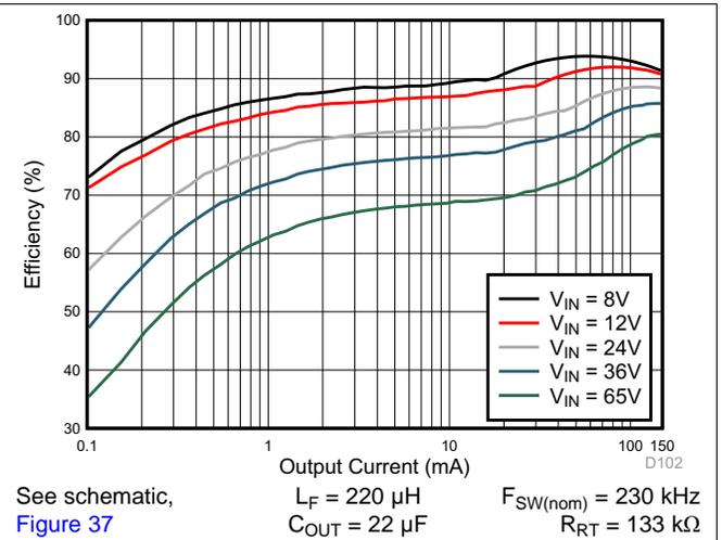
Figure 2. Converter Efficiency: 5 V, 150 mA, COT
