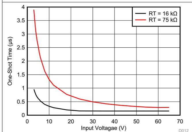
Figure 17. COT One-Shot Timer  $T_{ON}$  vs Input Voltage
