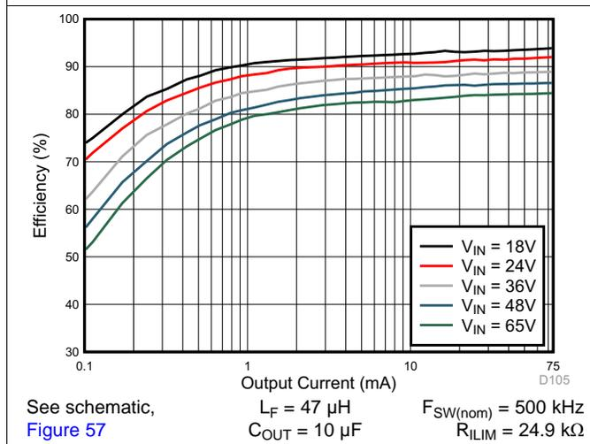
Figure 5. Converter Efficiency: 12 V, 75 mA, PFM
