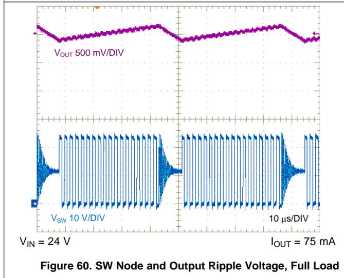
Figure 60. SW Node and Output Ripple Voltage, Full Load
