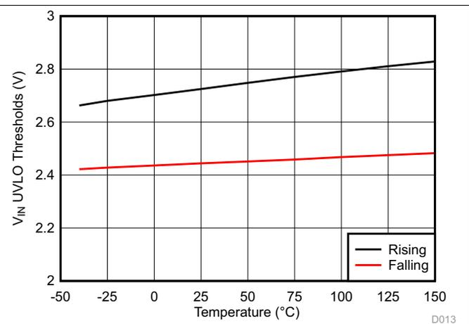
Figure 18. Internal  $V_{IN}$  UVLO Voltage vs Temperature
