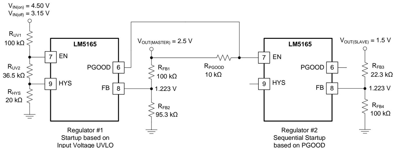
**Figure 36. Master-Slave Sequencing Implementation Using PGOOD and EN**
