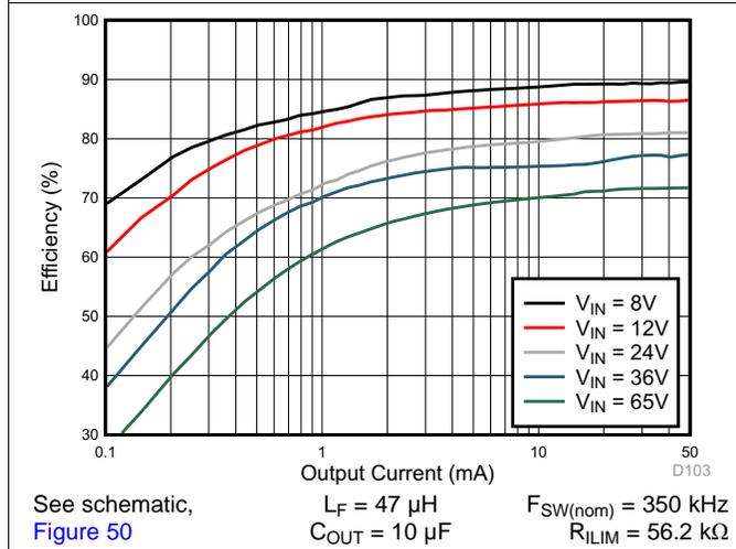
Figure 3. Converter Efficiency: 3.3 V, 50 mA, PFM
