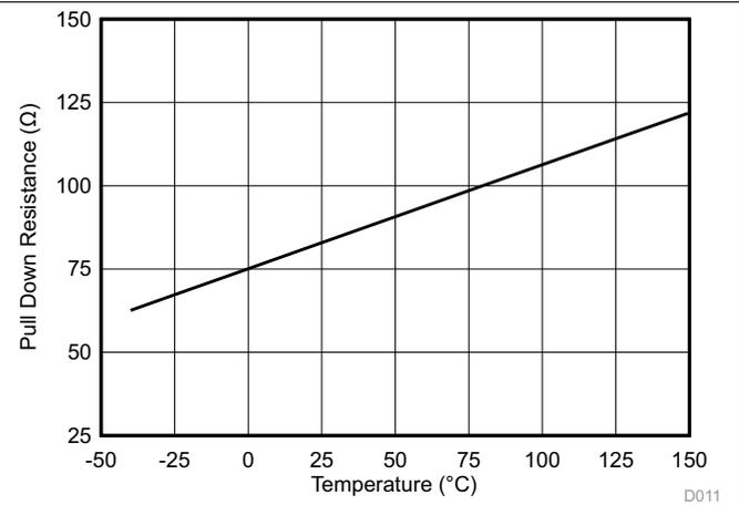
Figure 16. PGOOD and HYS Pulldown  $R_{DS(on)}$  vs Temperature
