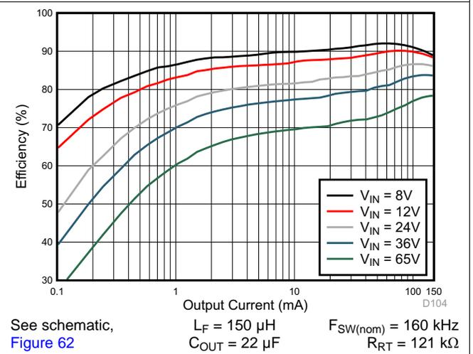
Figure 4. Converter Efficiency: 3.3 V, 150 mA, COT
