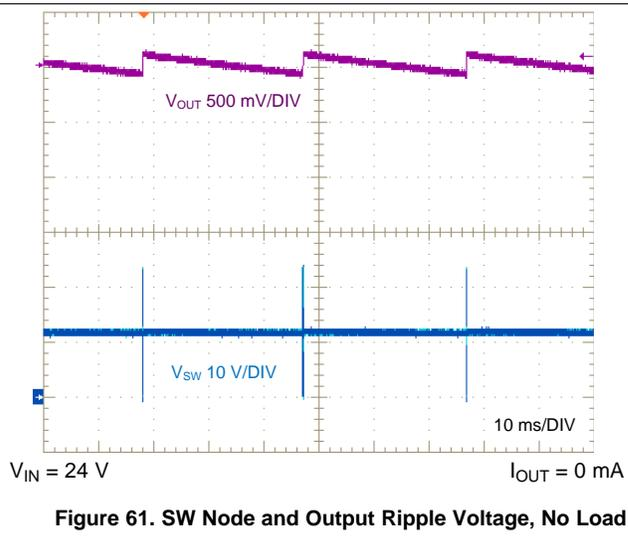
Figure 61. SW Node and Output Ripple Voltage, No Load
