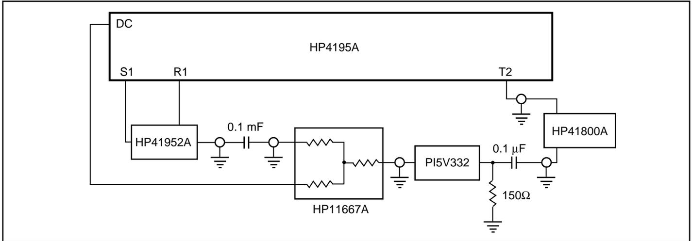
Figure 1. Differential Gain/Phase
