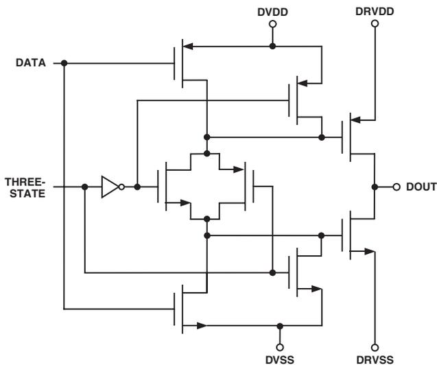
Figure 2. Data Outputs—D0–D11
