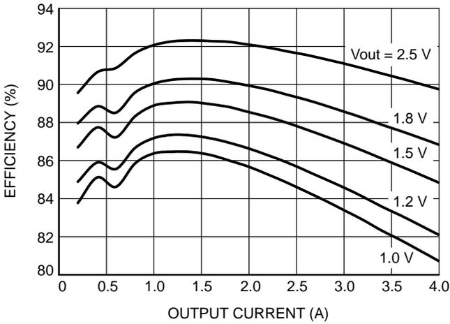
Figure 6. Efficiency at Auto CCM/DCM Mode
