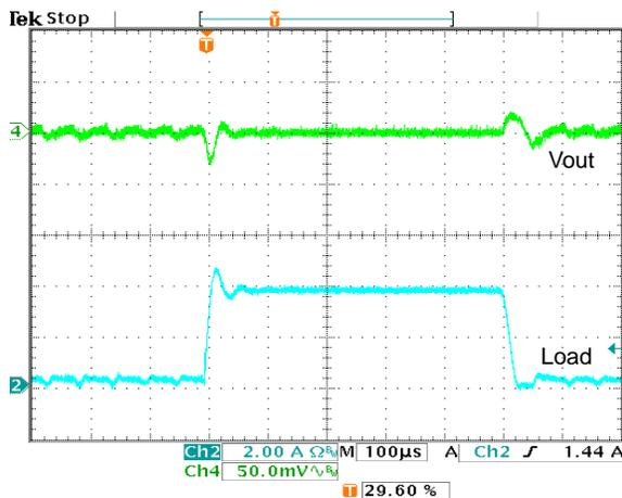
Figure 18. Load Transient at Auto CCM/DCM Mode
