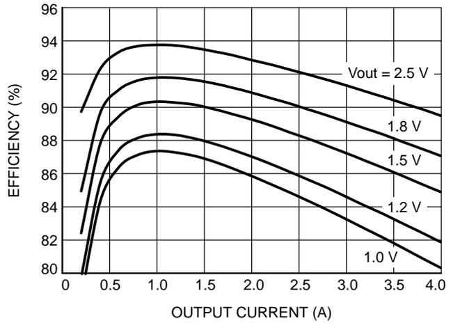
Figure 5. Efficiency at FCCM mode Vin = 3.3 V
