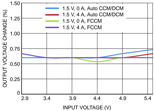
Figure 9. Line Regulation (input voltage vs. output voltage)
