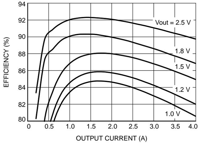
Figure 7. Efficiency at FCCM Mode Vin = 5.0 V
