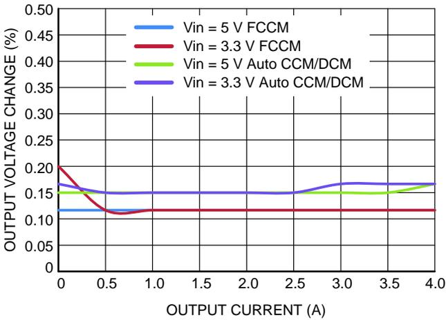
Figure 8. Load Regulation (output current vs. output voltage)
