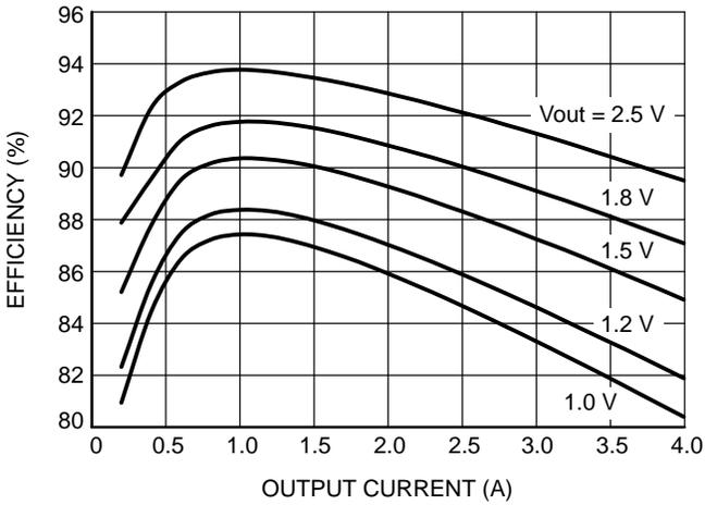
Figure 4. Efficiency at Auto CCM/DCM Mode
