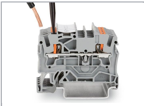
Insert fine-stranded conductors via operating tool.
