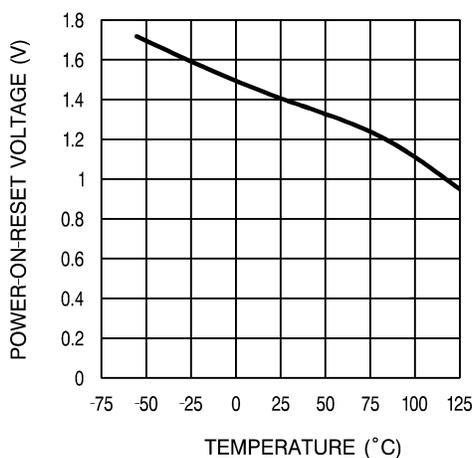
Figure 6. Average Power on Reset Voltage vs Temperature
