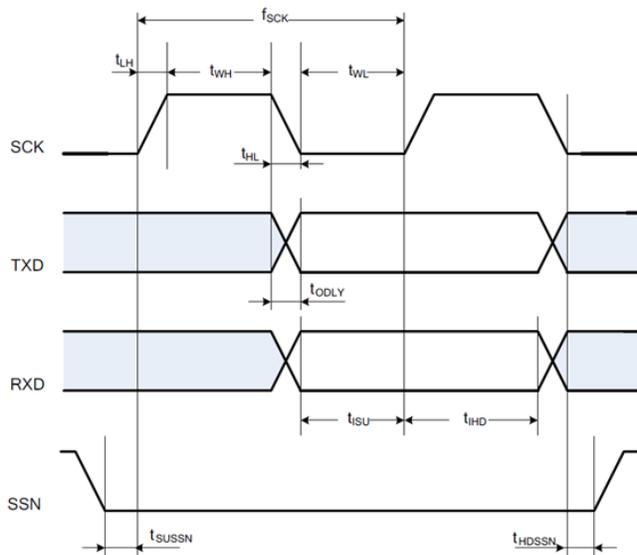
Table 10-6. ATWINC3400-MR210 SPI Slave Timing Parameters
