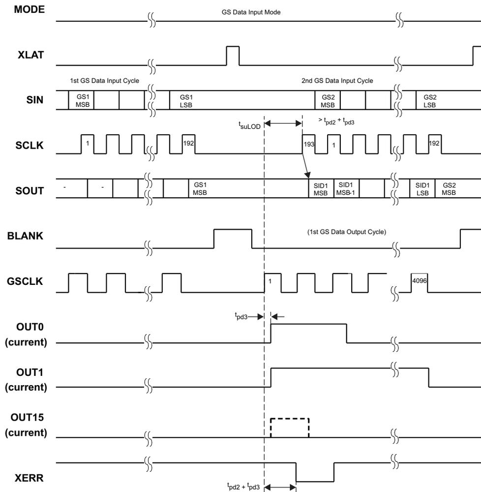
Figure 14. Readout Status Information Data (SID) Timing Chart
