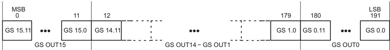
Figure 11. Grayscale Data Packet Format
