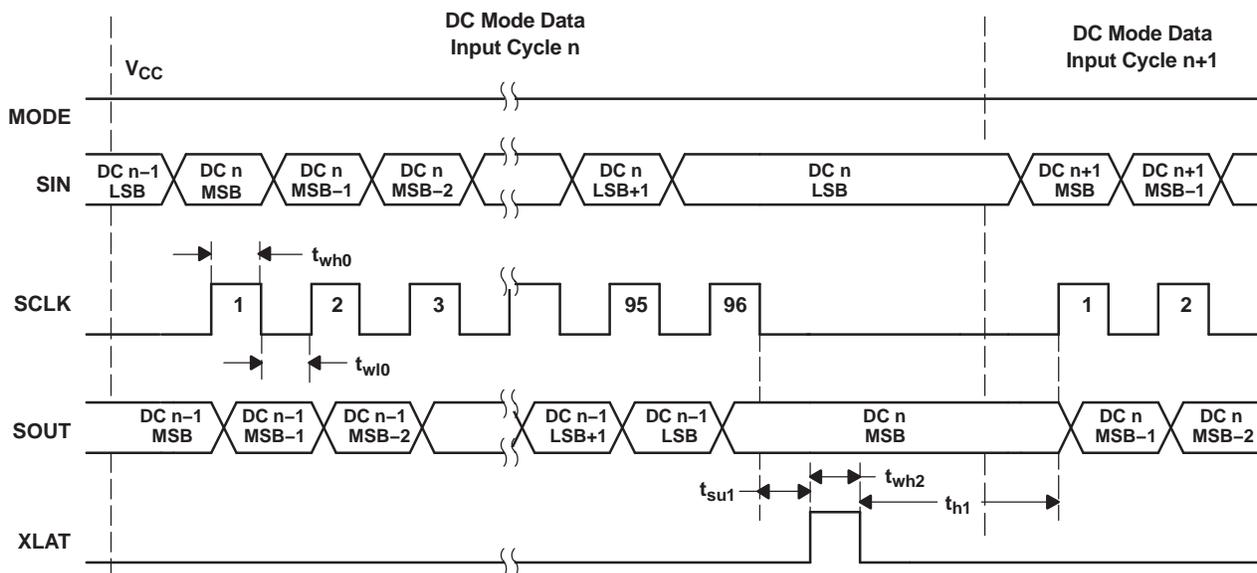
Figure 10. Dot Correction Data Input Timing Chart
