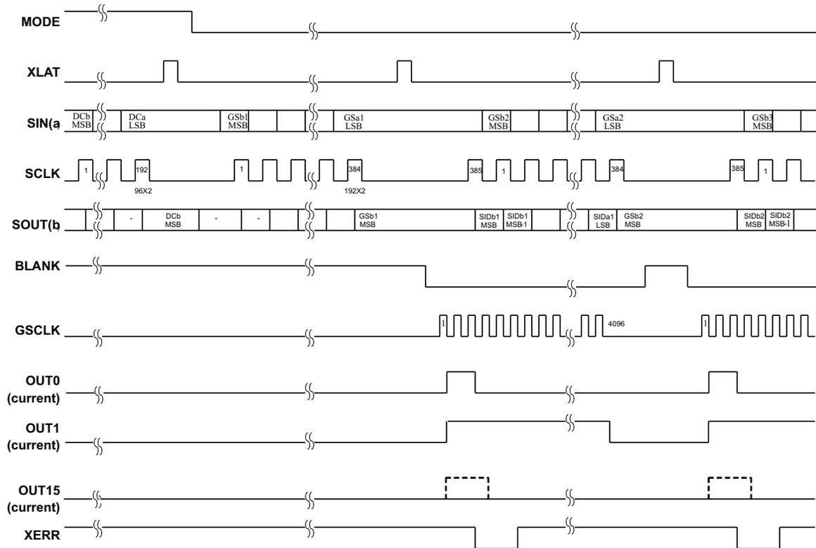
Figure 8. Timing Chart for Two Cascaded TLC5945 Devices
