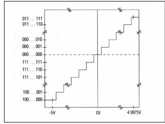
Figure 17. Bipolar Transfer Function
