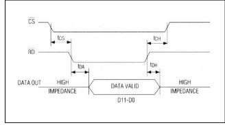
Figure 6. Data-Access and Bus-Relinquish Timing
