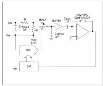
Figure 4. Equivalent Input Circuit
