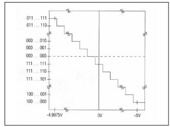
Figure 21. Inverting Bipolar Transfer Function
