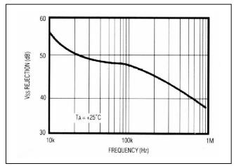
Figure 15. V<sub>SS</sub> Power-Supply Rejection vs. Frequency
