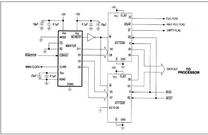
Figure 13. Using MAX120 with FIFO Memory
