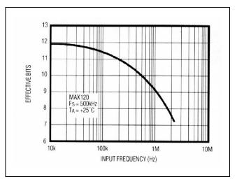
Figure 23. Effective Bits vs. Input Frequency
