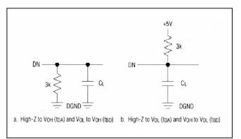
Figure 2. Load Circuits for Bus-Relinquish Time
