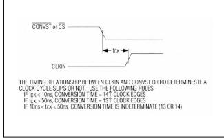
Figure 5. Clock and Control Synchronization
