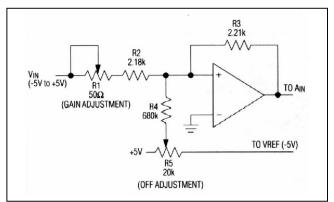
Figure 19. Offset and Gain Adjustment (Noninverting)
