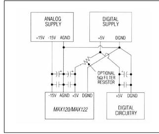
Figure 14. Power-Supply Grounding
