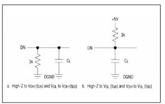
Figure 1. Load Circuits for Access Time
