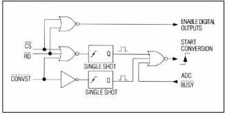
Figure 12. Conversion-Control Logic
