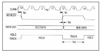
Figure 11. Continuous-Conversion Mode (Mode 5)
