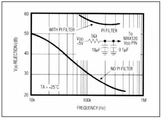
Figure 16. V<sub>DD</sub> Power-Supply Rejection vs. Frequency
