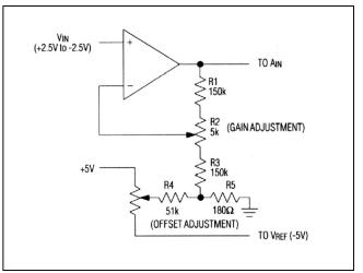
Figure 19. Offset and Gain Adjustment (Noninverting)
