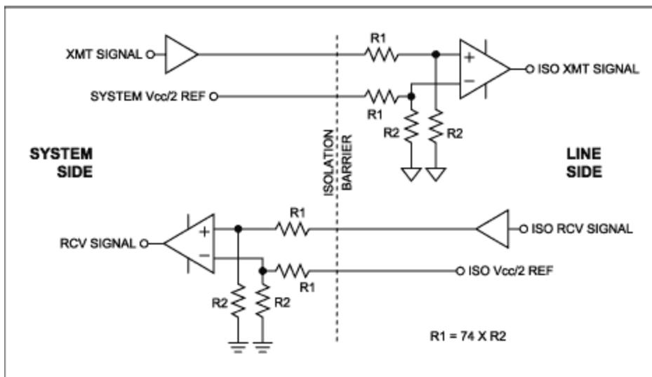
Figure 3. Resistive isolation technique.
