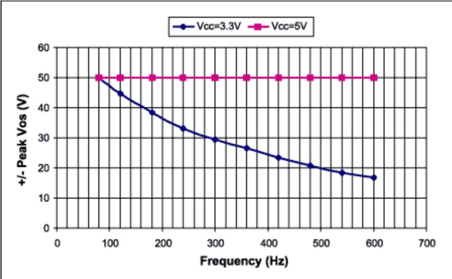
Figure 8. Maximum applied offset voltage vs. frequency for 3.3V and 5V operation.
