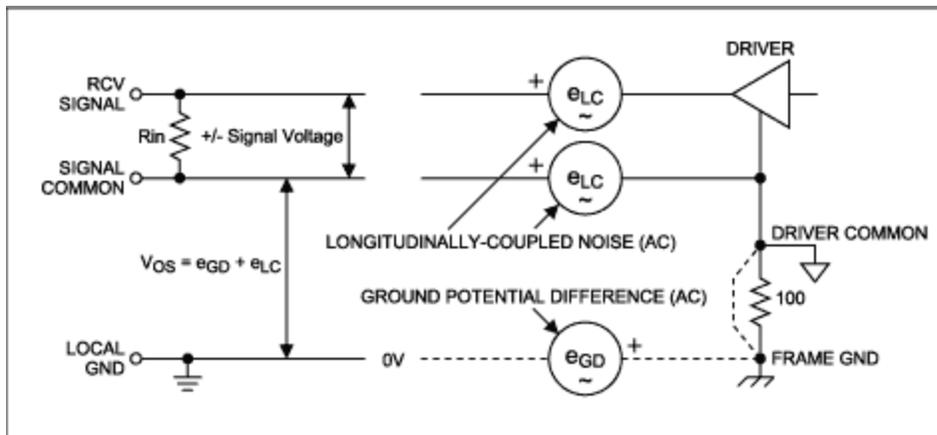
Figure 2. Offset voltages in two-wire line data-transmission system.
