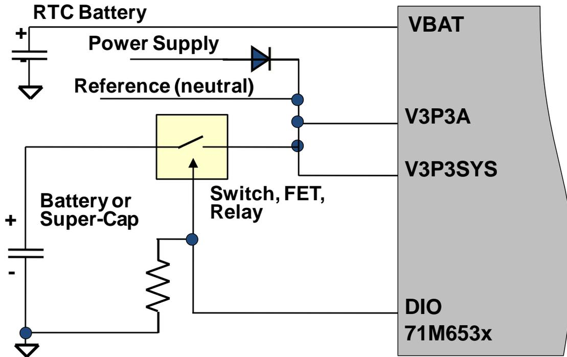
Figure 1: Sample Circuitry for Return to BSMM
