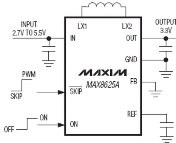
**Figure 2: Buck Boost Circuit with 3.3 VDC Output**
