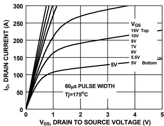
Figure 10. Saturation Characteristics
