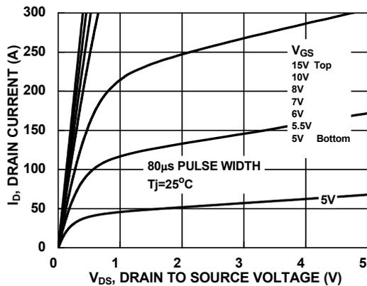
Figure 9. Saturation Characteristics
