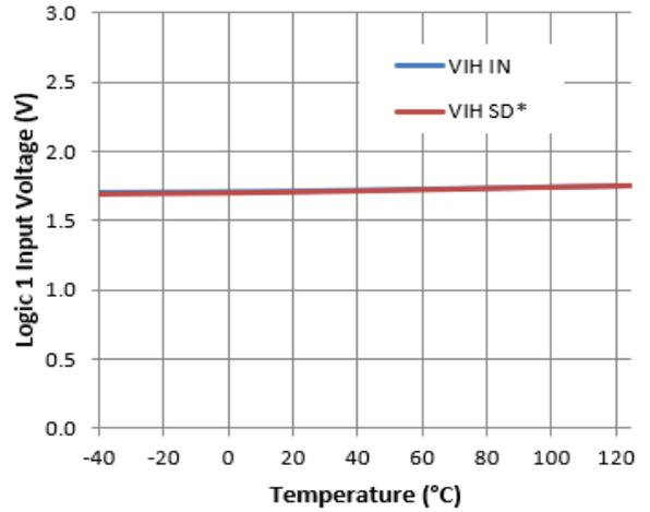
**Figure 23.** Logic 1 Input Voltage vs. Temperature
