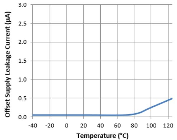
**Figure 31.** Offset Supply Leakage Current vs. Temperature
