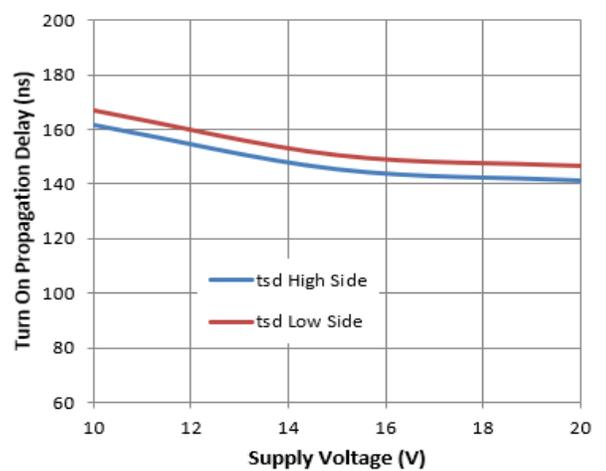
**Figure 9.** SD Propagation Delay vs. Supply Voltage
