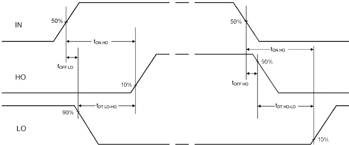
$t_{DT\ LO-HO} = t_{ON\ HO} - t_{OFF\ LO}$
