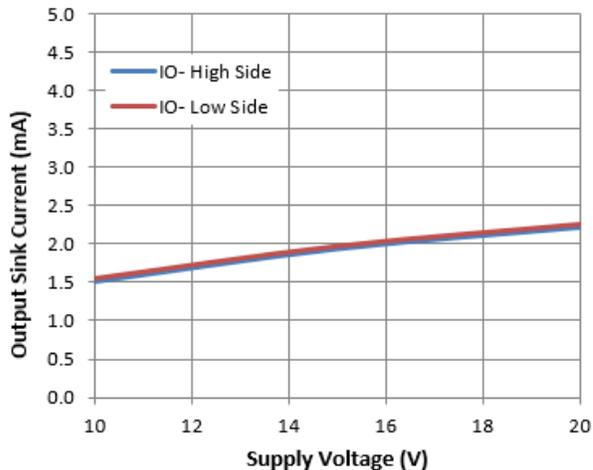
**Figure 20.** Output Sink Current vs. Supply Voltage
