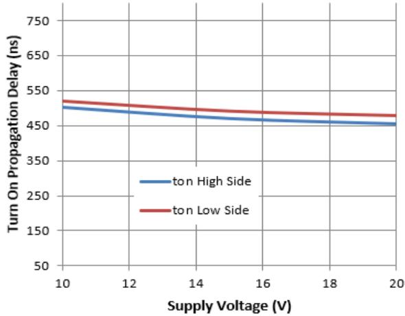
**Figure 4.** Turn-on Propagation Delay vs. Supply Voltage
