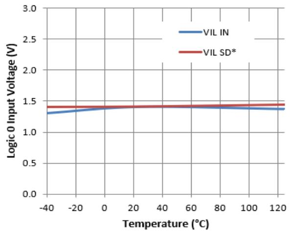
**Figure 25.** Logic 0 Input Voltage vs. Temperature
