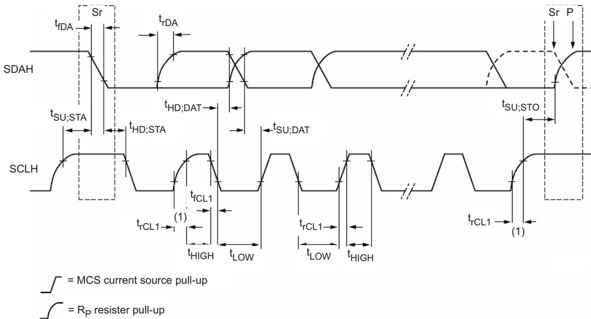
Figure 33. Serial Interface Timing for H/S Mode
