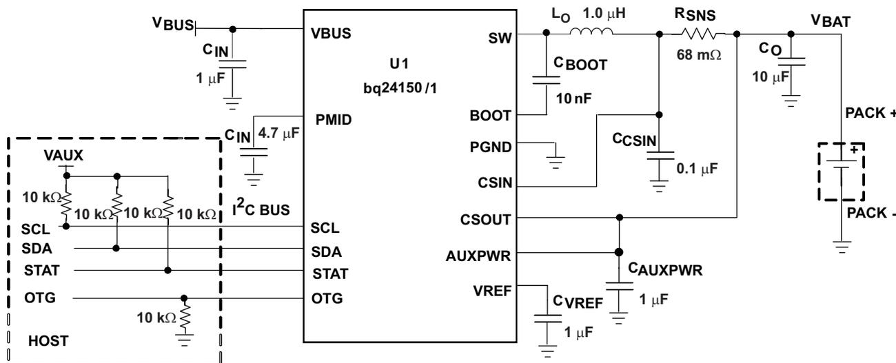
Figure 1. I<sup>2</sup>C Controlled 1-Cell Charger Application Circuit
