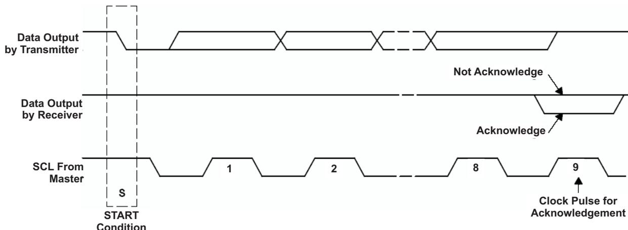
Figure 29. Acknowledge on the I<sup>2</sup>C Bus™
