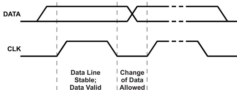
**Figure 28. Bit Transfer on the Serial Interface**
