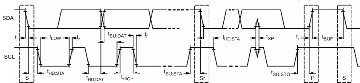
Figure 32. Serial Interface Timing for F/S Mode
