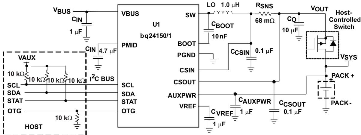
Figure 2. I<sup>2</sup>C Controlled 1-Cell Pre-Regulator Application
