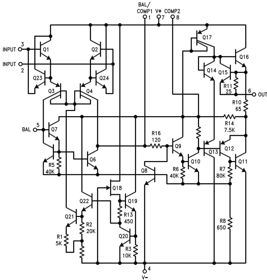
Pin connections shown are for 8-pin packages.
