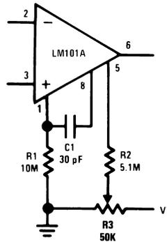
Figure 38. Standard Compensation and Offset Balancing Circuit
