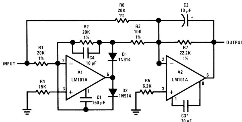
Feedforward compensation can be used to make a fast full wave rectifier without a filter.
