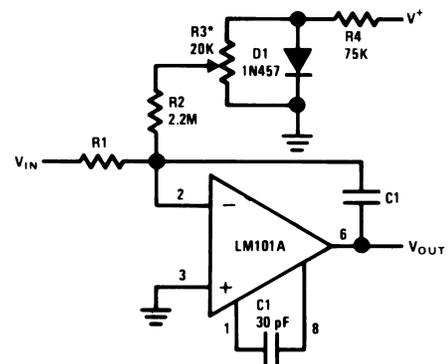
\*Adjust for zero integrator drift. Current drift typically 0.1 nA/°C over -55°C to +125°C temperature range.
