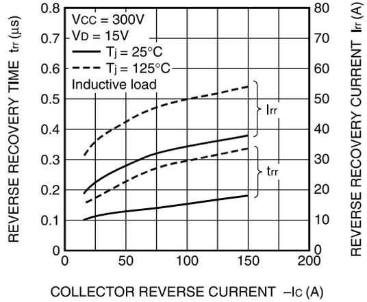
**SWITCHING RECOVERY LOSS CHARACTERISTICS (TYPICAL)**
