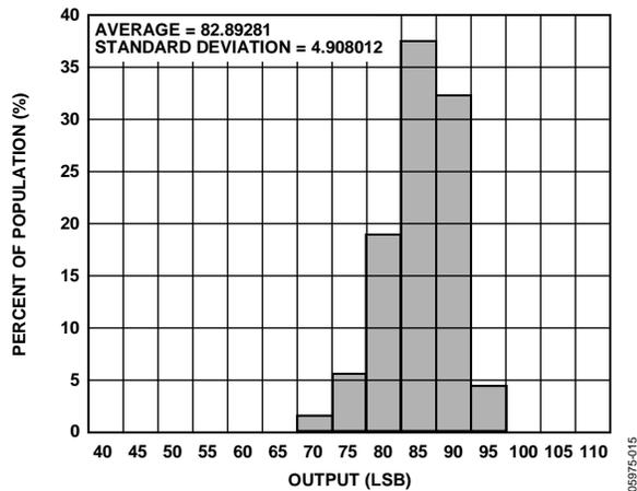
Figure 15. X-Axis Self-Test at  $V_{CC} = 3.3\text{ V}$ ,  $25^\circ\text{C}$
