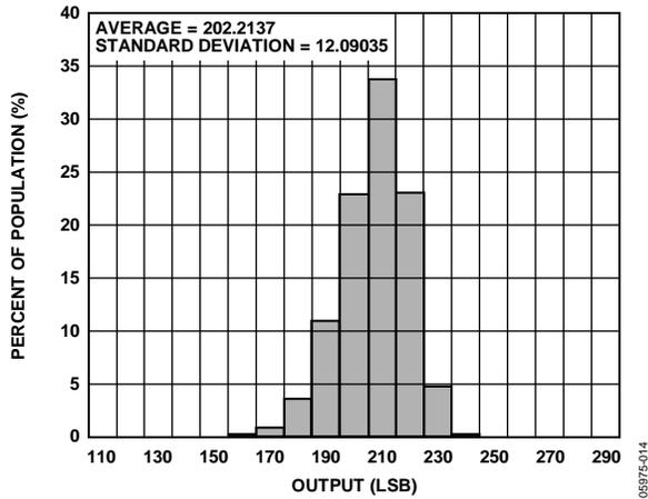
Figure 14. X-Axis Self-Test at  $V_{CC} = 5\text{ V}$ ,  $25^\circ\text{C}$
