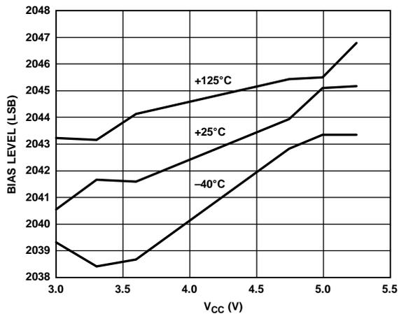
Figure 9. X-Axis 0 g Bias vs. Supply Voltage
