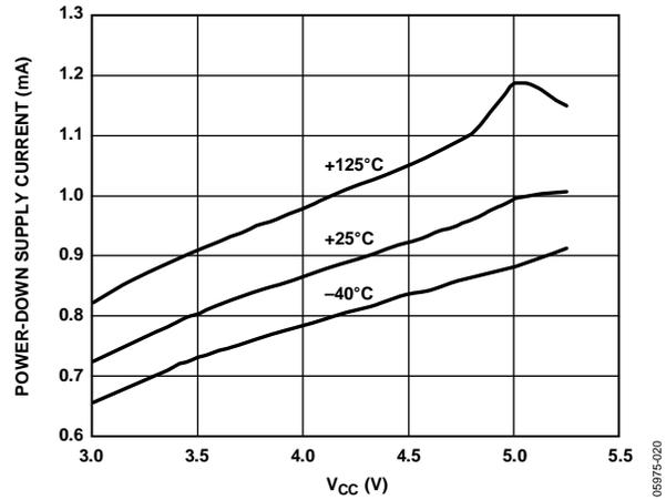
Figure 21. Power-Down Supply Current vs. Supply Voltage
