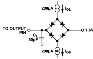
Figure 2. Load Circuit for Digital Output Timing Specifications
