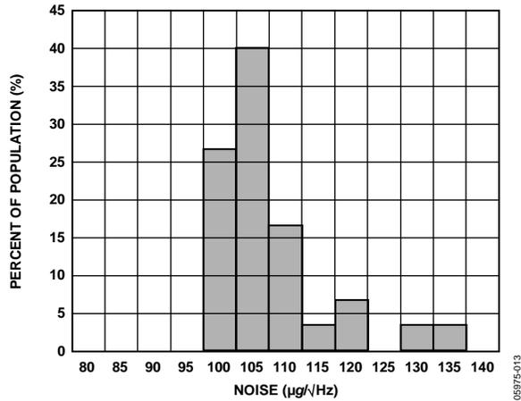
Figure 13. Noise (Y-Axis) at  $V_{CC} = 5\text{ V}$ ,  $25^\circ\text{C}$
