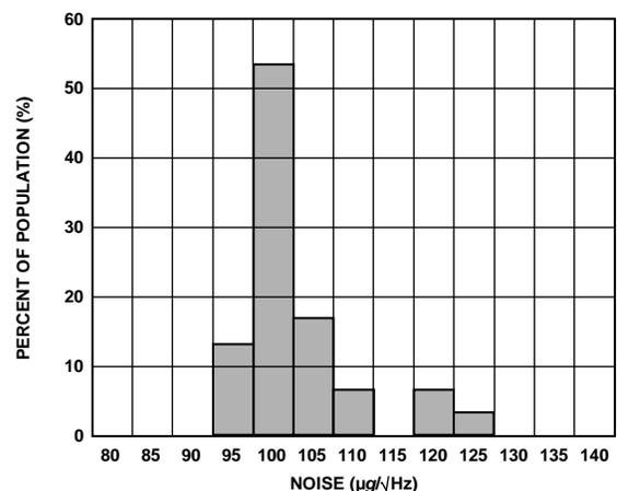
Figure 12. Noise (X-Axis) at V<sub>CC</sub> = 5 V, 25°C
