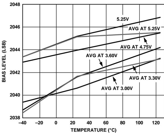
Figure 8. X-Axis 0 g Bias vs. Temperature
