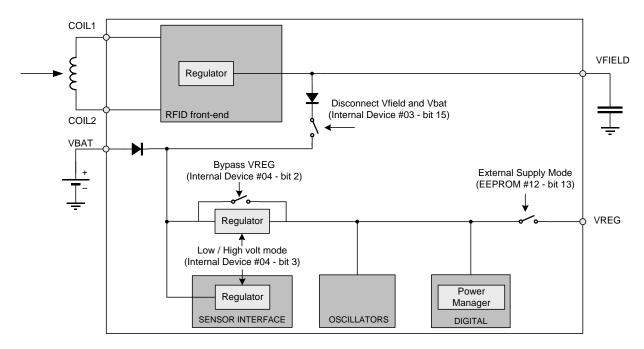
The power management mode is defined by several switches configurable through the EEPROM and EE-Latch.
