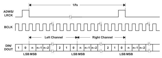
Figure 17. Timing Diagram for DSP Mode
