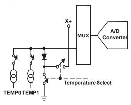
Figure 25. Functional Block Diagram of Temperature Measurement Mode
