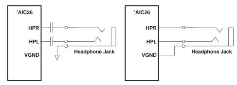
Figure 21. Headphone Configurations, AC-Coupled (left) and Capless (right)
