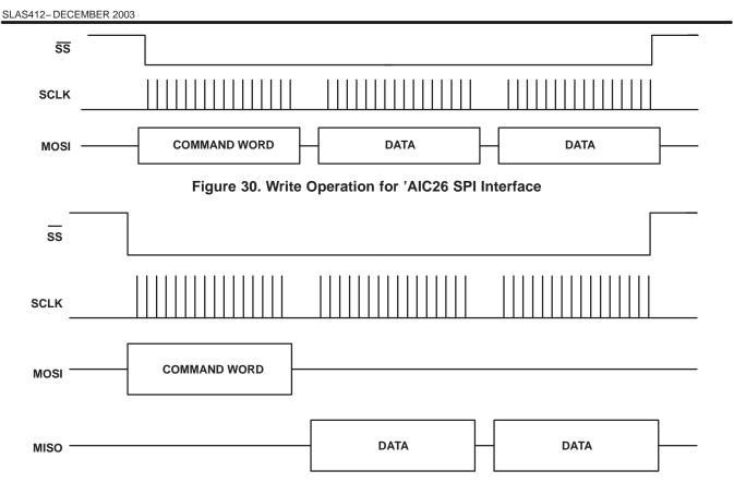
Figure 31. Read Operation for 'AIC26 SPI Interface
