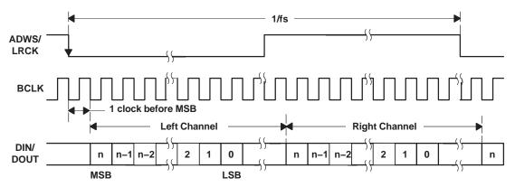
Figure 16. Timing Diagram for I<sup>2</sup>S Mode
