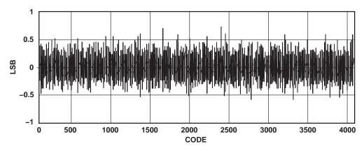
Figure 6. SAR DNL ( $T_A = 25$ °C, Internal Ref = 2.5 V, AVDD = 3.3 V)
