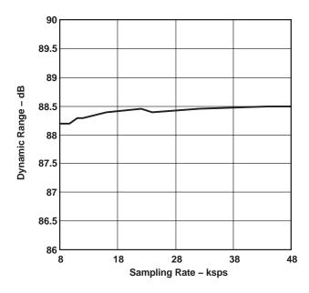
Figure 9. ADC Dynamic Range vs Sampling Speed ( $T_A = 25$ °C, AVDD = 3.3 V)
