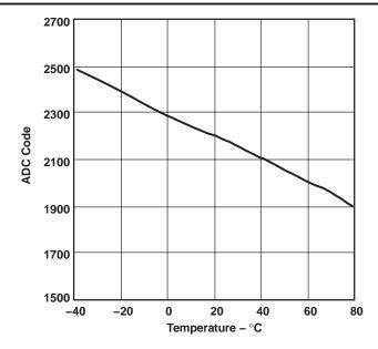
Figure 26. Typical Plot for Single Measurement Method
