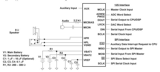
Figure 13. Typical Circuit Configuration
