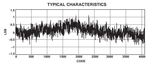
Figure 5. SAR INL ( $T_A = 25$ °C, Internal Ref = 2.5 V, 12 bit, AVDD = 3.3 V)
