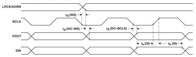
Figure 1. I<sup>2</sup>S/LJF/RJF Timing in Master Mode
