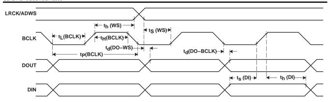
Figure 3. I<sup>2</sup>S/LJF/RJF Timing in Slave Mode
