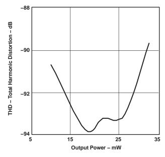
Figure 12. High Power Output Driver THD vs Output Power (T\_A =25°C, AVDD, DRVDD = 3.3 V, R\_L = 16  $\Omega$ )
