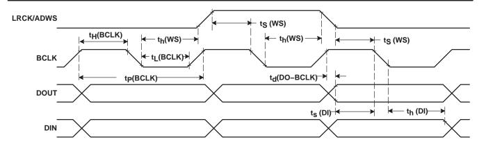
Figure 4. DSP Timing in Slave Mode
