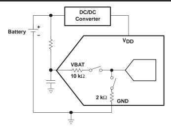
Figure 28. Battery Measurement Functional Block Diagram
