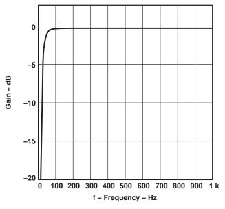
Figure 20. Frequency Response For 16- $\Omega$  Load and 50- $\mu$ F Decoupling Capacitor After Gain Compensation Using a Suggested Set of Coefficients for Audio Effects Filter
