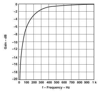
Figure 19. Uncompensated Response For 16- $\Omega$  Load and 50- $\mu$ F Decoupling Capacitor
