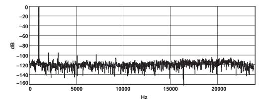
Figure 8. ADC FFT Plot at 48 ksps ( $T_A = 25^{\circ}C$ , -1 dB, 1 kHz Input, AVDD = 3.3 V)
