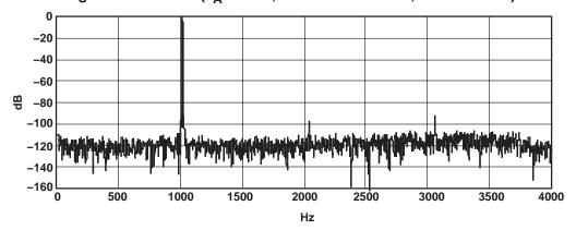
Figure 7. ADC FFT Plot at 8 ksps ( $T_A = 25^{\circ}C$ , -1 dB, 1 kHz Input, AVDD = 3.3 V)
