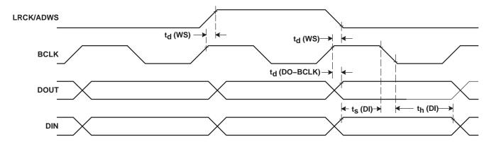
Figure 2. DSP Timing in Master Mode
