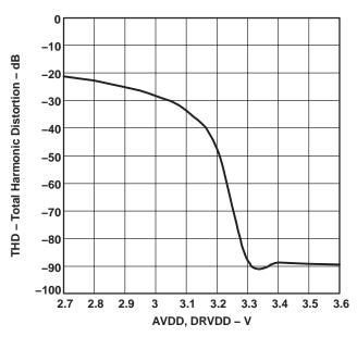
Figure 24. THD vs AVDD, DRVDD Supply Voltage (25°C When Driving a –1 dB, 1-kHz Sinewave From the DAC Into an 8-Ω Load, with DAC Output Swing Set to 2.4 V, and Short-Circuit Protection Disabled)
