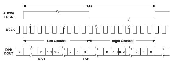
Figure 14. Timing Diagram for Right-Justified Mode
