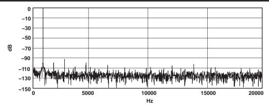
Figure 11. DAC FFT Plot (T<sub>A</sub> = 25°C, 48 ksps, –1 dB, 1 kHz Input, AVDD = DRVDD = 3.3 V, DVDD = 1.8 V, R<sub>L</sub> = 16  $\Omega$ )
