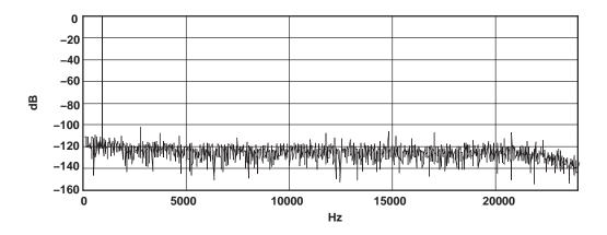
Figure 10. DAC FFT Plot (T<sub>A</sub> = 25°C, 48 ksps, 0 dB, 1 kHz Input, AVDD = 3.3 V, R<sub>L</sub> = 10 k $\Omega$ )
