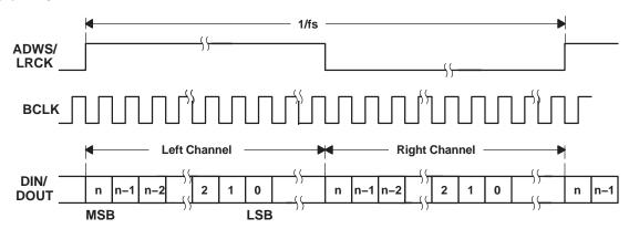
Figure 15. Timing Diagram for Left-Justified Mode
