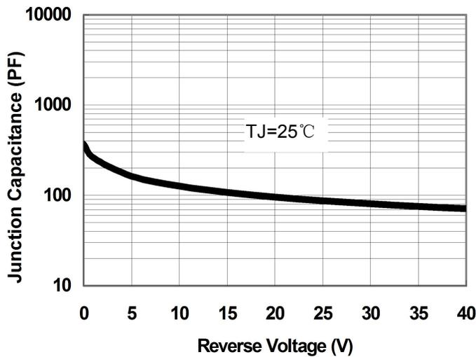
Fig.1-Typical Junction Capacitance
