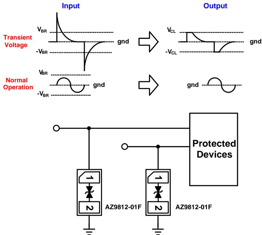
Fig. 1 ESD protection scheme by using AZ9812-01F.
