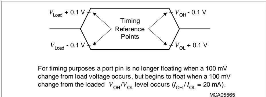
**Figure 18 Floating Waveforms**
