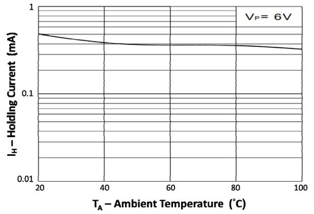
Fig 8 Holding Current vs Ambient Temperature
