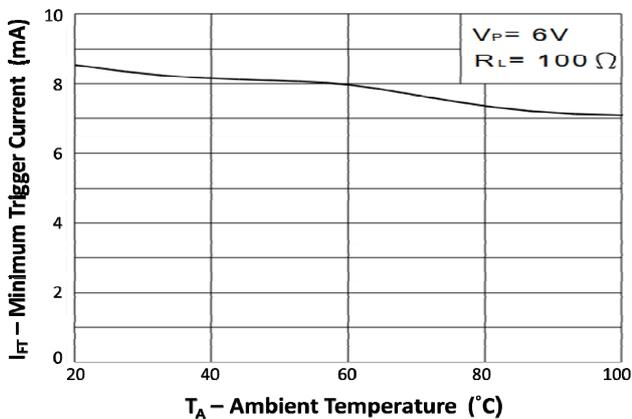
Fig 5 Minimum Trigger Current vs Ambient Temperature
