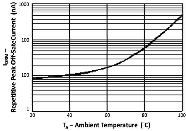
Fig 7 Repetitive Peak Off-State Current vs Ambient Temperature
