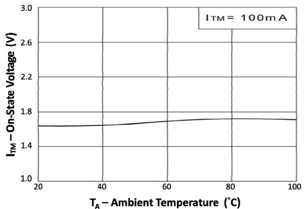
Fig 6 On-State Voltage vs Ambient Temperature
