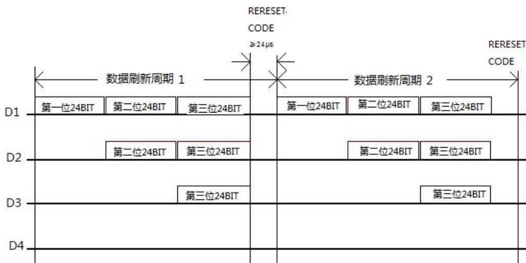
Notes: D1 is the MCU terminal transmission data, D2, D3, D4 is Cascade circuit automatic forwarding data.
