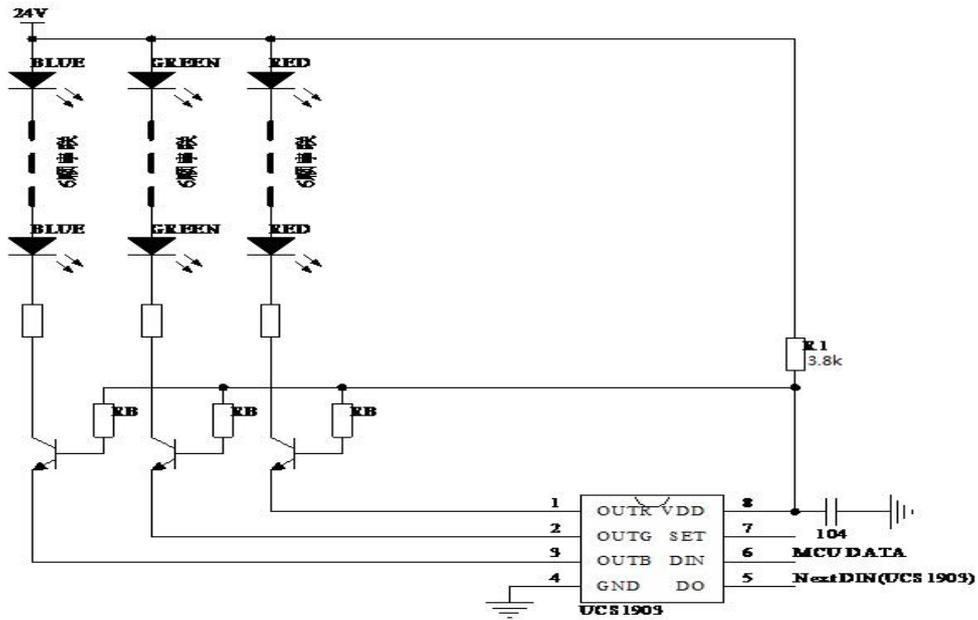
UCS1903 Power Supply Voltage can configuration 6—24V, 104p capacitance should to close IC, Resistance configuration according to different voltage. The below is resistance listed:
