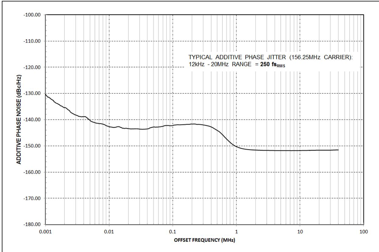
**FIGURE 5-2:** Typical Additive Phase Jitter: 156.25 MHz Carrier, 12 kHz to 20 MHz Range, 250 fs<sub>RMS</sub>.
