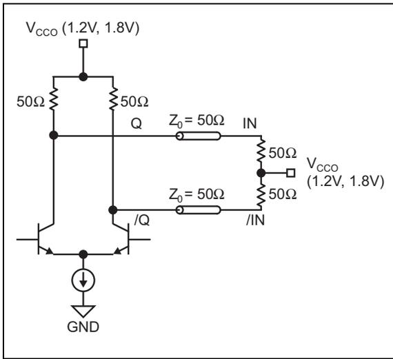
**FIGURE 8-1:** 1.2V or 1.8V CML DC-Coupled Termination.
