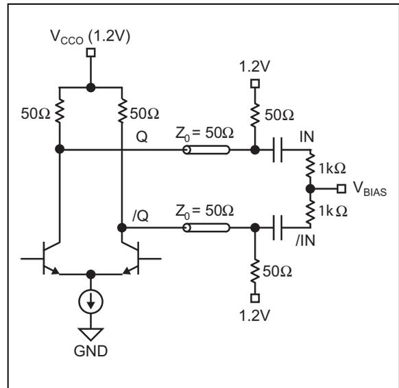
**FIGURE 8-4:** CML AC-Coupled Termination ( $V_{CCO}$  1.2V Only).
