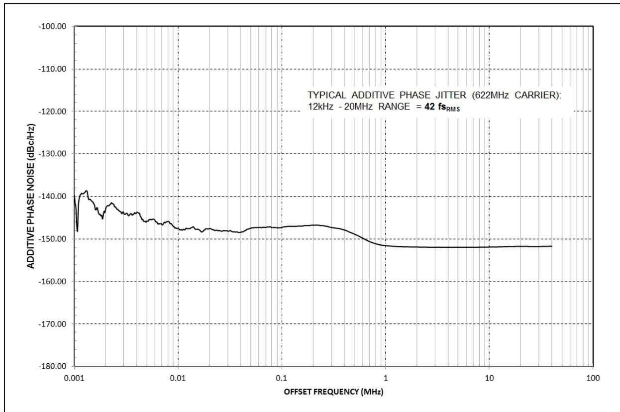
**FIGURE 5-1:** Typical Additive Phase Jitter: 622 MHz Carrier, 12 kHz to 20 MHz Range, 42 fs<sub>RMS</sub>.
