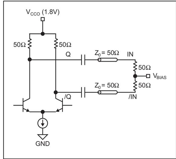
**FIGURE 8-3:** CML AC-Coupled Termination ( $V_{CCO}$  1.8V Only).
