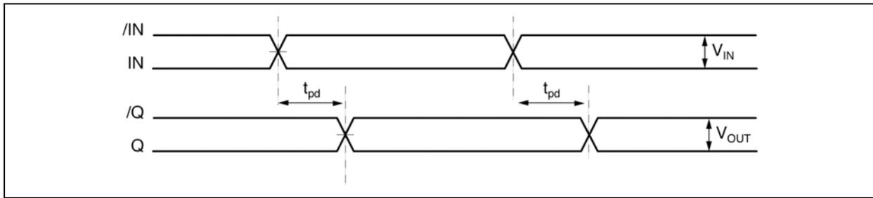
**FIGURE 6-1:** Propagation Delay.
