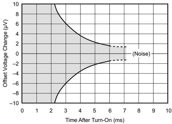
Figure 6-9. Input-Referred Offset Voltage WarmUp
