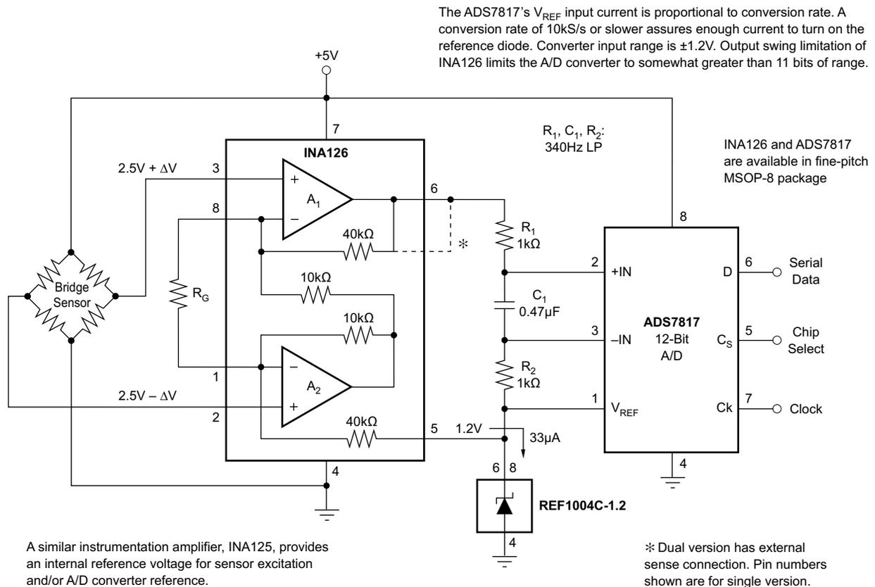
**Figure 9-1. Bridge Signal Acquisition, Single 5-V Supply**
