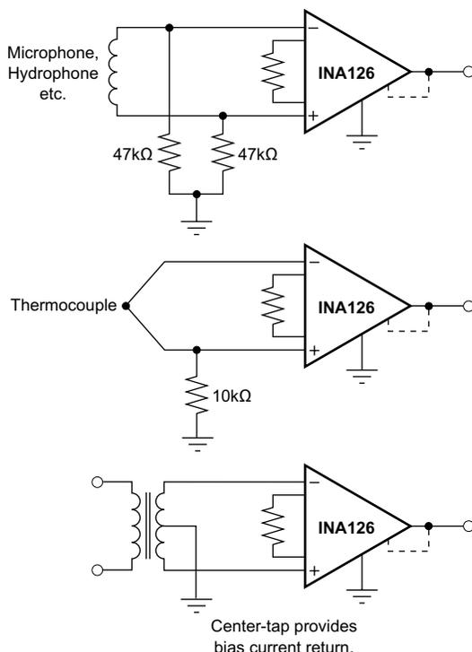
**Figure 8-3. Providing an Input Common-Mode Current Path**
