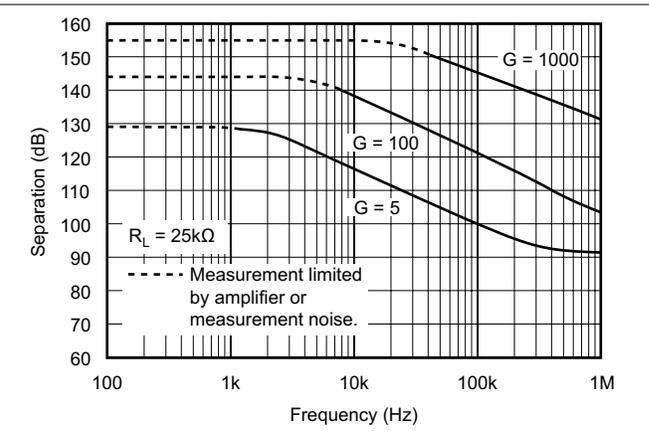
**Figure 6-18. Channel Separation vs Frequency, RTI (Dual Version)**
