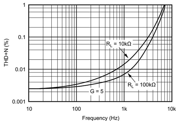
Figure 6-12. Total Harmonic Distortion + Noise vs Frequency
