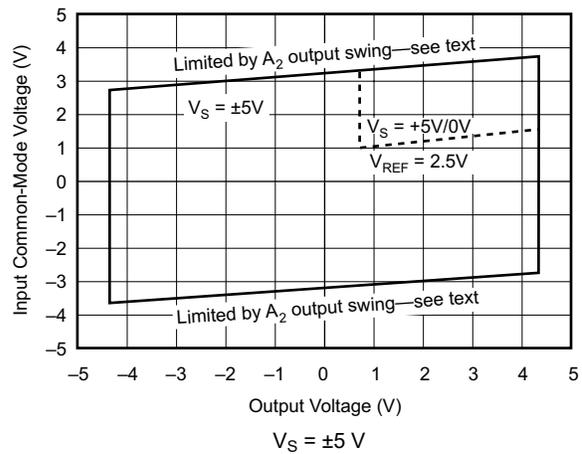
Figure 6-6. Input Common-Mode Voltage Range vs Output Voltage
