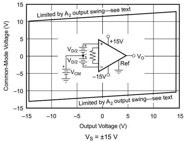
Figure 6-5. Input Common-Mode Voltage Range vs Output Voltage
