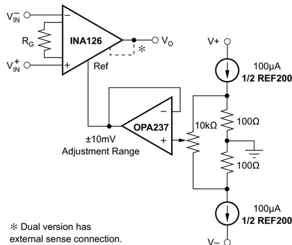
**Figure 8-2. Optional Trimming of Output Offset Voltage**
