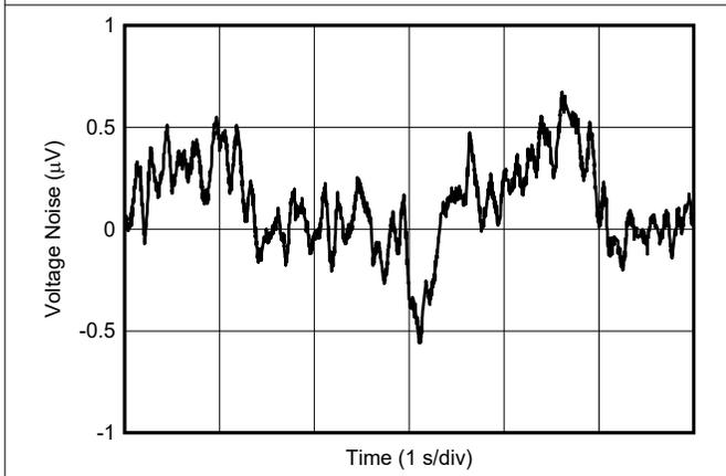
**Figure 6-17. 0.1-Hz to 10-Hz Voltage Noise**
