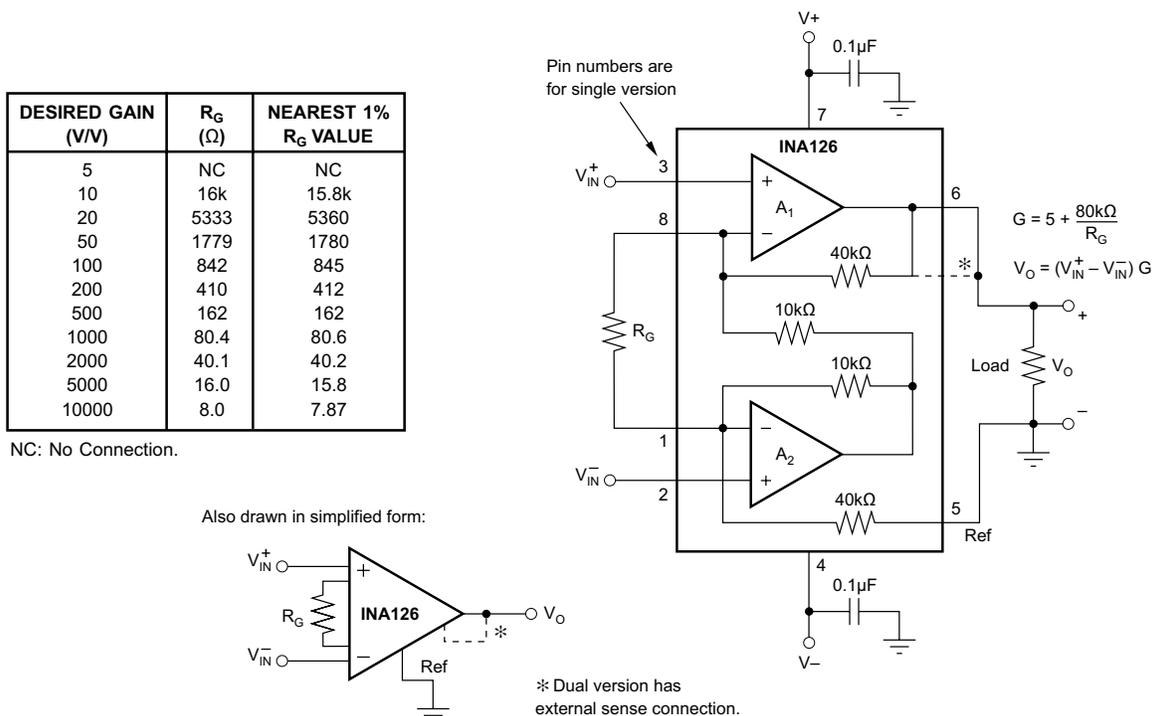
Figure 8-1. Basic Connections
