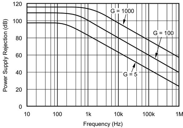
Figure 6-3. Positive Power Supply Rejection vs Frequency
