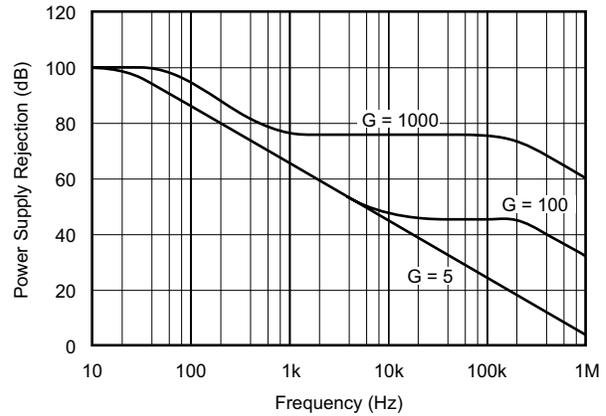
Figure 6-4. Negative Power Supply Rejection vs Frequency
