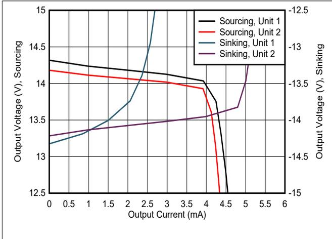
**Figure 6-13. Output Voltage Swing vs Output Current**
