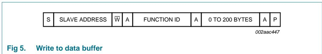
Fig 5. Write to data buffer
