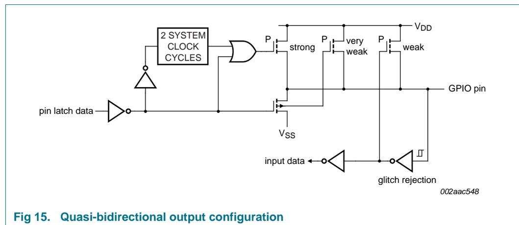
**Fig 15. Quasi-bidirectional output configuration**
