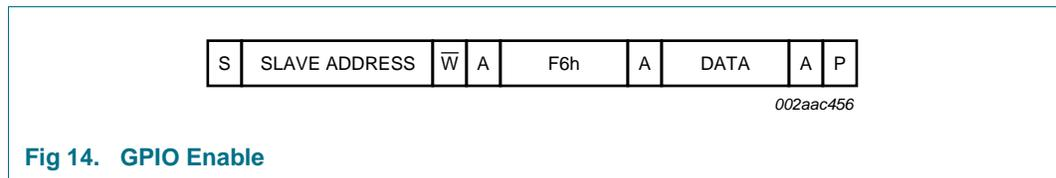
Fig 14. GPIO Enable
