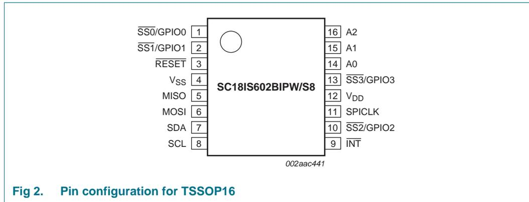
Fig 2. Pin configuration for TSSOP16
