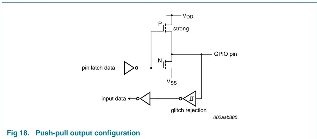
Fig 18. Push-pull output configuration
