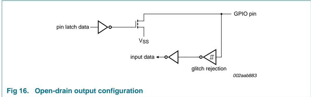
Fig 16. Open-drain output configuration
