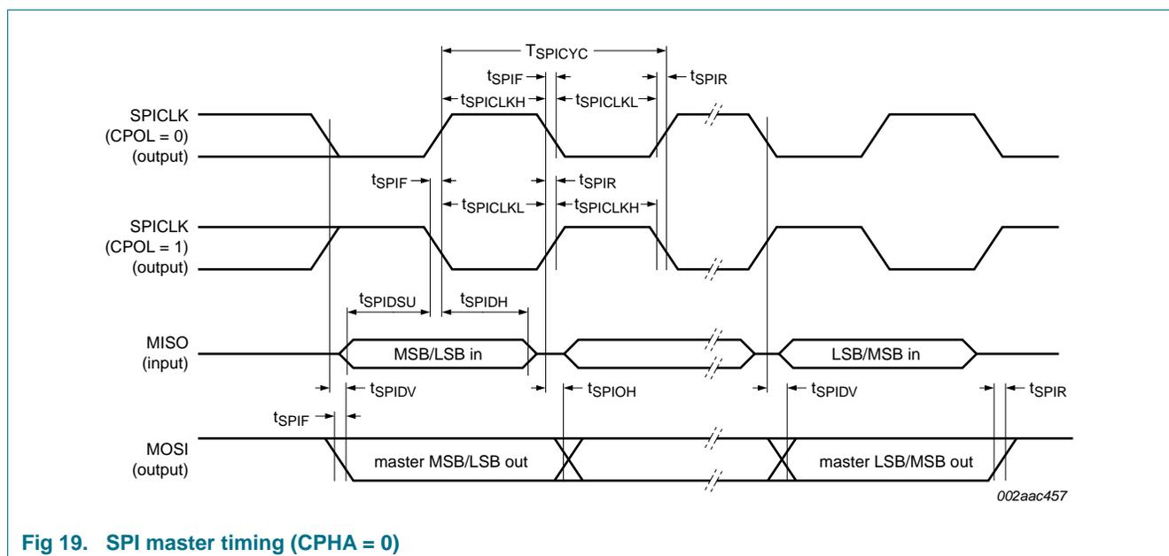
**Fig 19. SPI master timing (CPHA = 0)**
