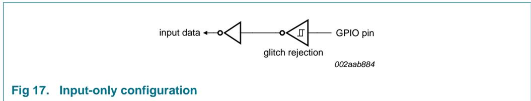
Fig 17. Input-only configuration
