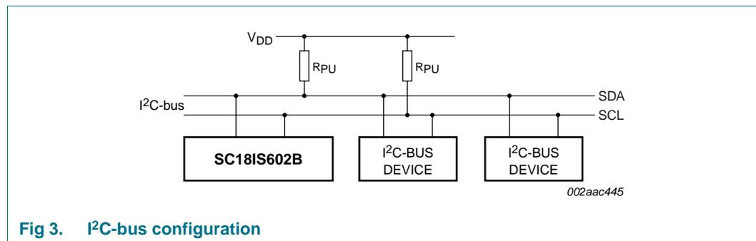
**Fig 3. I<sup>2</sup>C-bus configuration**
