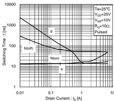
Fig.8 Switching Characteristics
