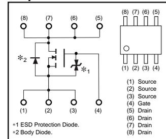
\* A protection diode is included between the gate and the source terminals to protect the diode against static electricity when the product is in use. Use a protection circuit when the fixed voltage are exceeded.
