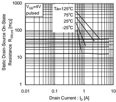
Fig.4 Static Drain-Source On-State Resistance vs. Drain Current (3)
