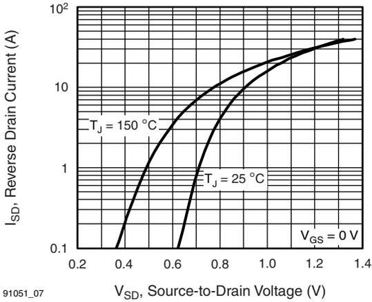
Fig. 6 - Typical Source-Drain Diode Forward Voltage
