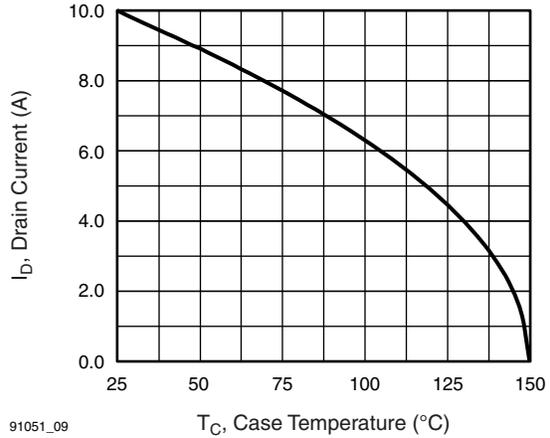
Fig. 8 - Maximum Drain Current vs. Case Temperature
